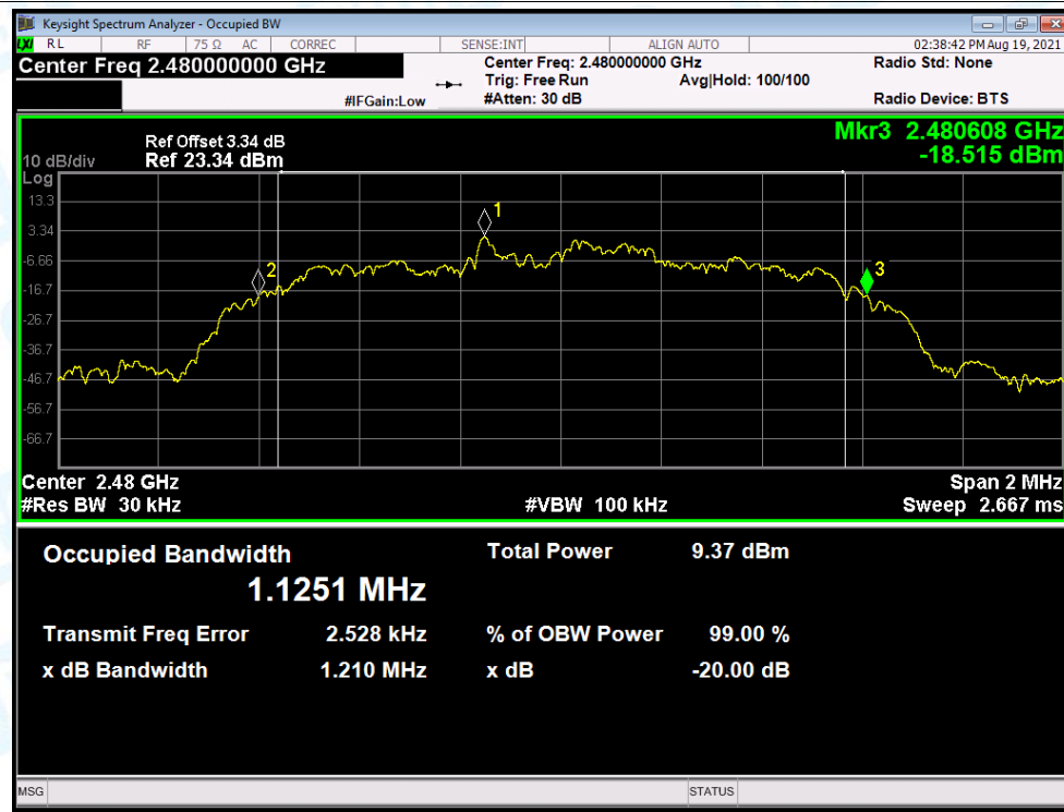
-20dB Bandwidth NVNT 2-DH1 2480MHz Ant1
