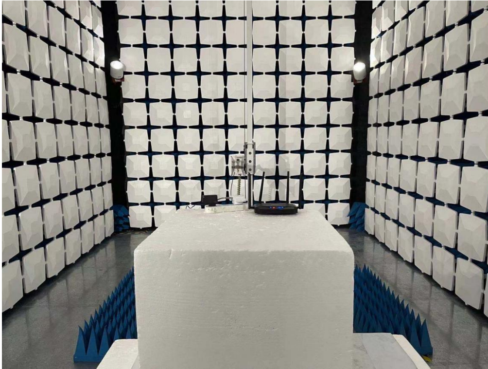
Above 1GHz for radiated emission test setup
