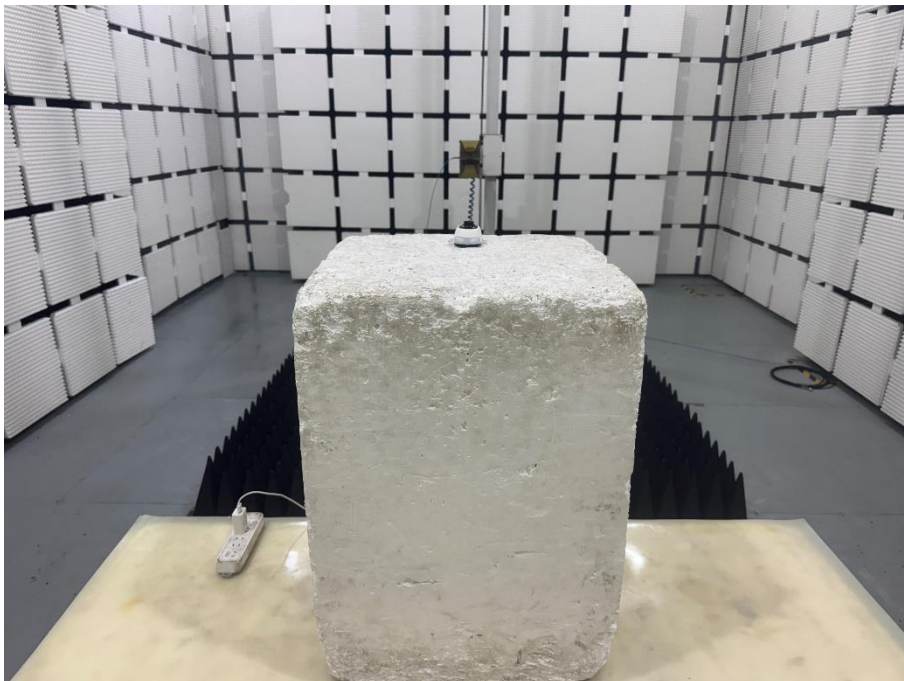
Set-up for Radiated Spurious Emission, Above 1GHz
