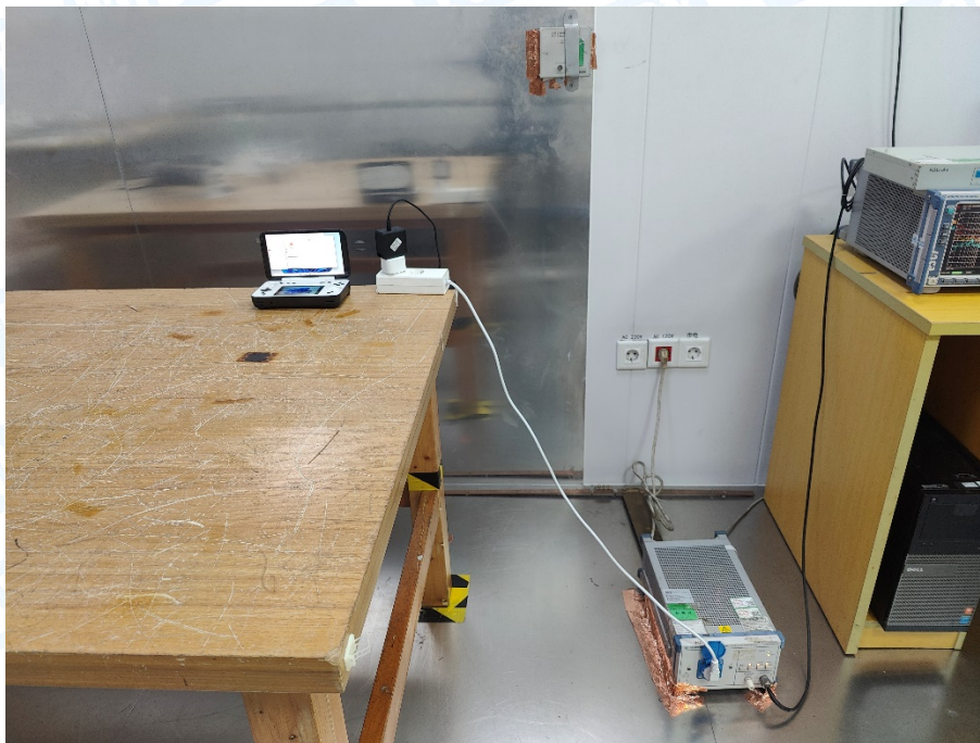
Photo of Setup for Conducted Emission
