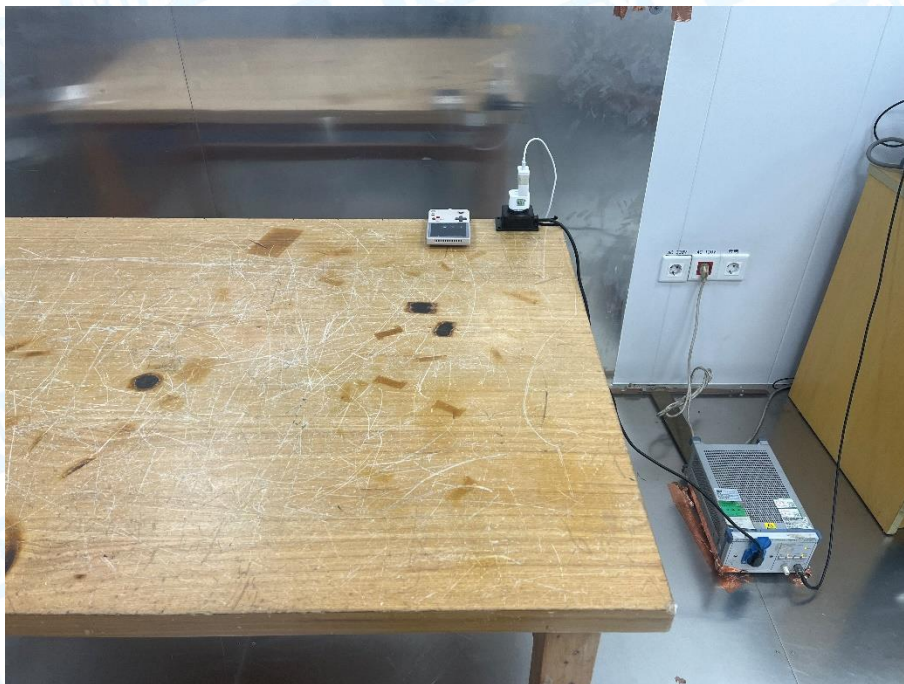
Photo of Setup for Conducted Emission
