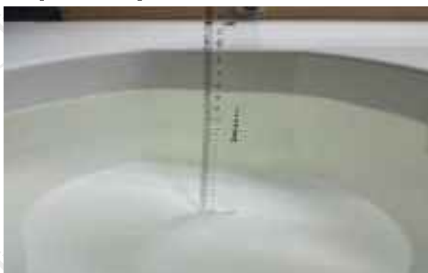
The Body Liquid of 2450MHz (15.3cm)
