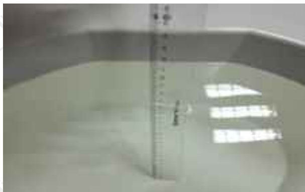
The Body Liquid of 5000-6000MHz (16.5cm)
