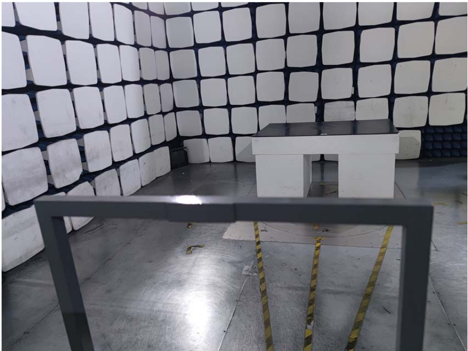
Radiation Emission Test Setup (Below 30MHz)
