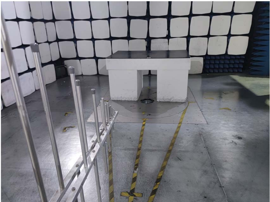
Radiation Emission Test Setup (30MHz to 1GHz)
