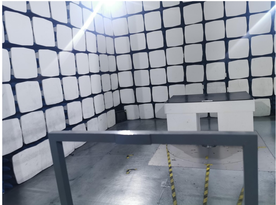
Radiation Emission Test Setup (Below 30MHz)
