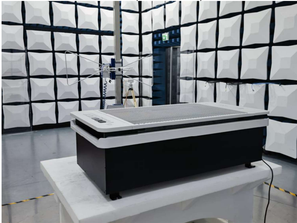
Radiated Emission (30 MHz – 1 GHz) – EUT B
