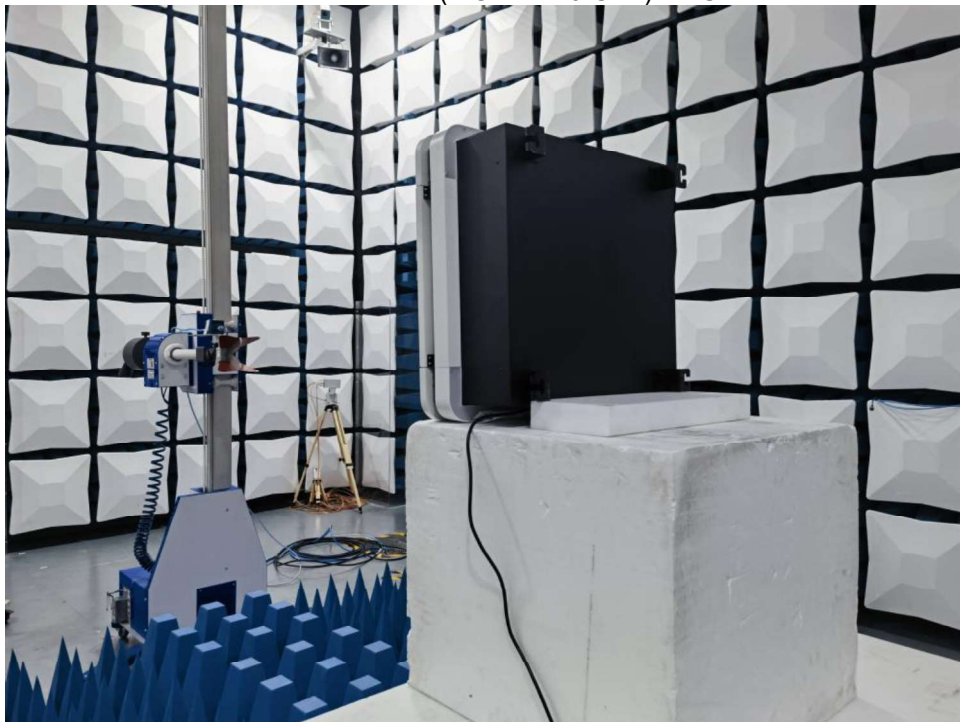
Radiated Emission (1 GHz – 40 GHz) – EUT B
