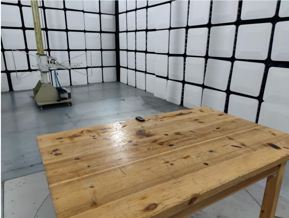
Photo of Radiation Emission Test
