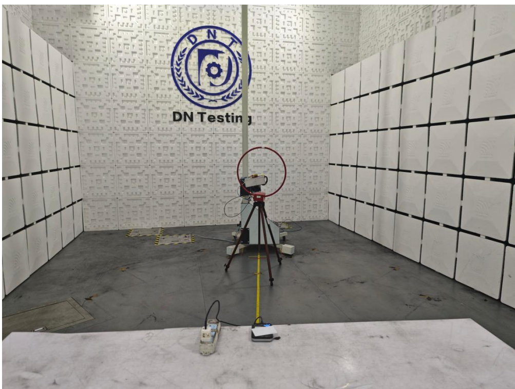
Radiated Emission Test View(9KHz-30MHz)
