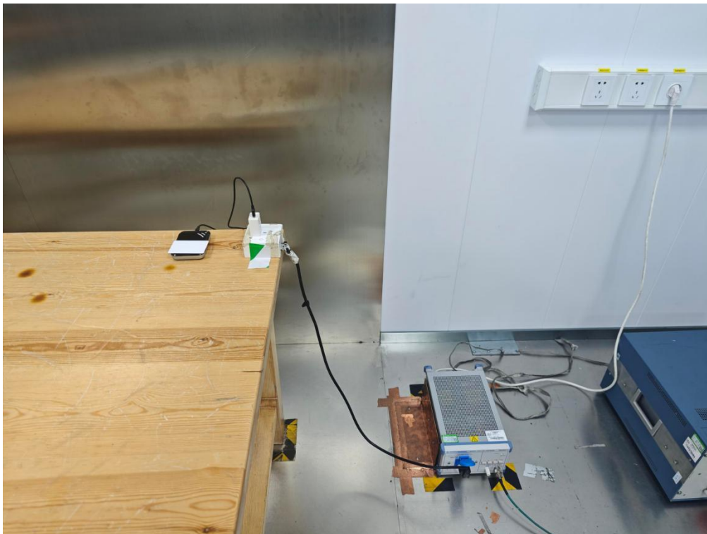
Radiated Emission Test View(9KHz-30MHz)
