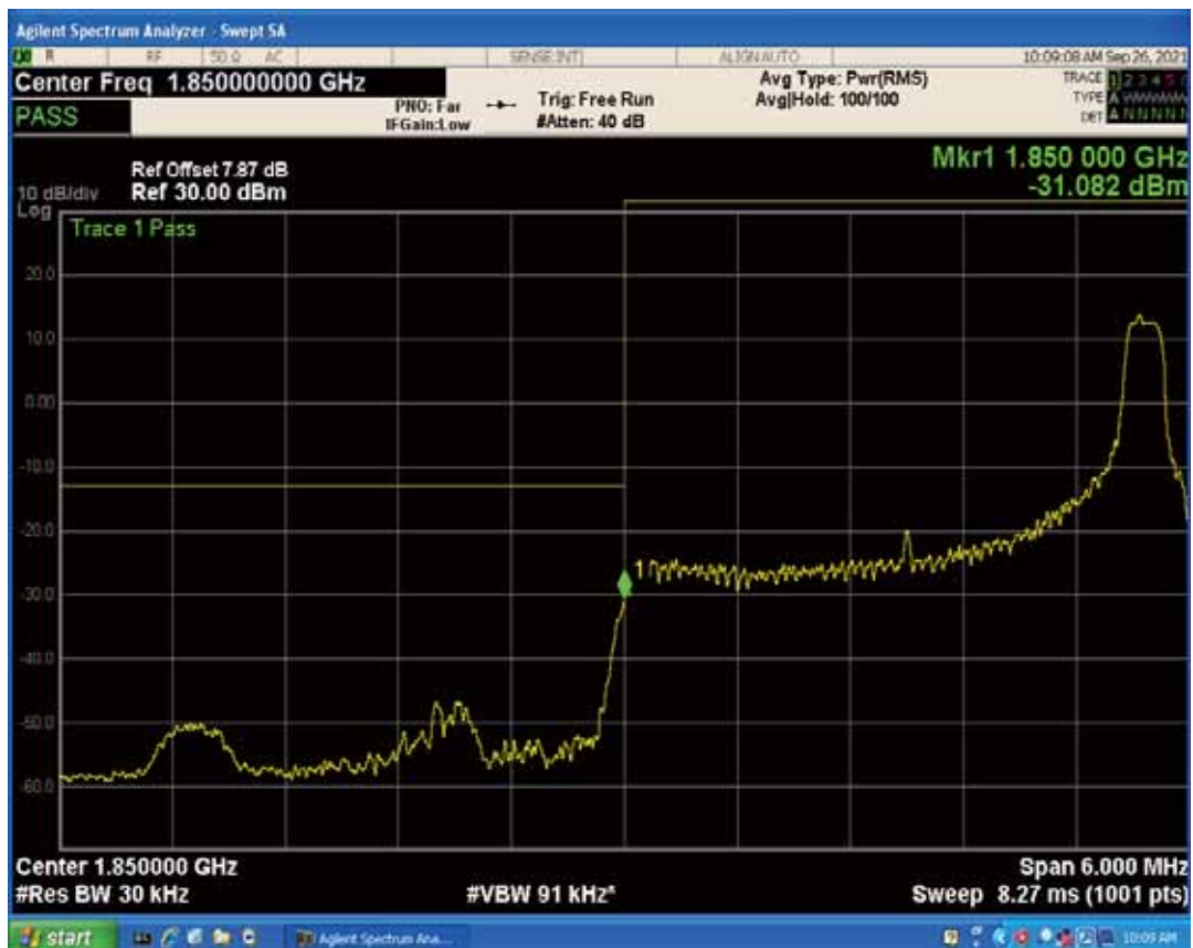
Band2 QAM16 BW=3MHz Channel=18615 RB Size=15 Position=#0
