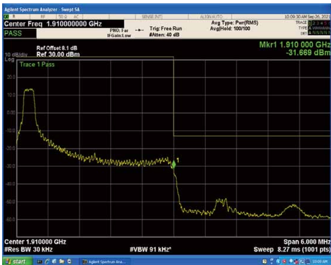
Band2 QAM16 BW=3MHz Channel=19185 RB Size=1 Position=#Max
