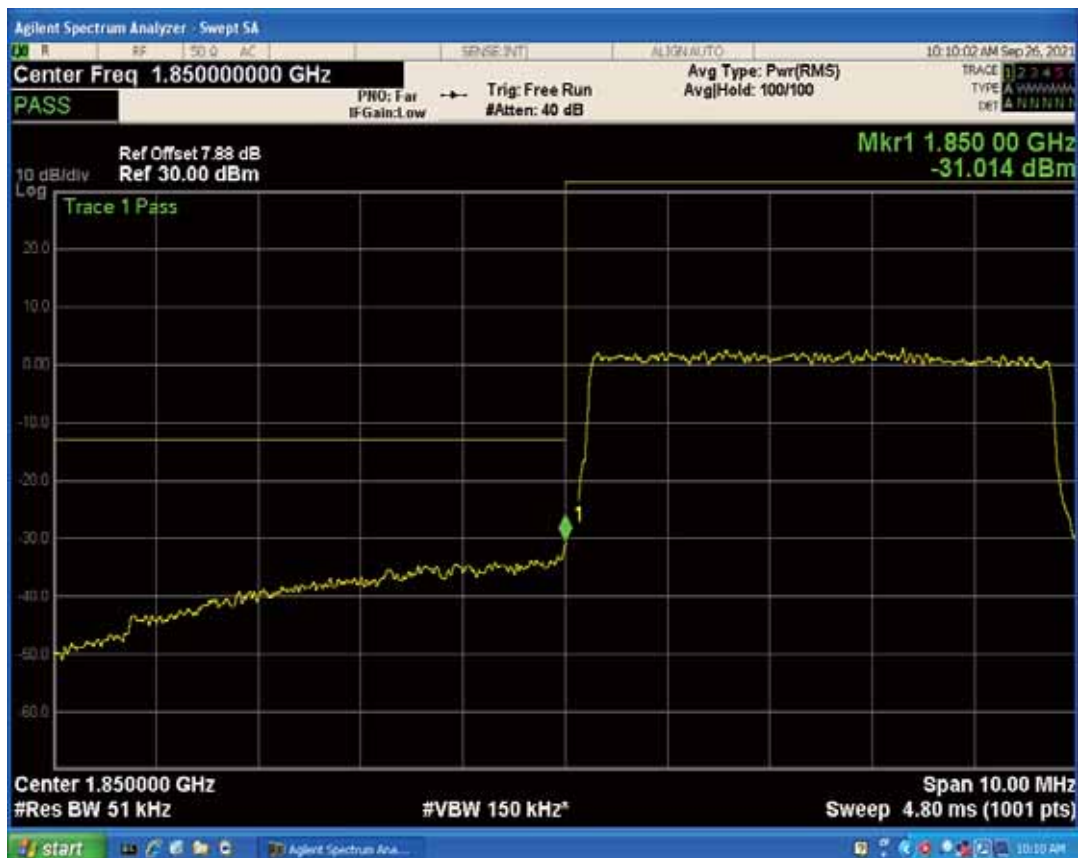
Band2 QAM16 BW=5MHz Channel=18625 RB Size=1 Position=#0
