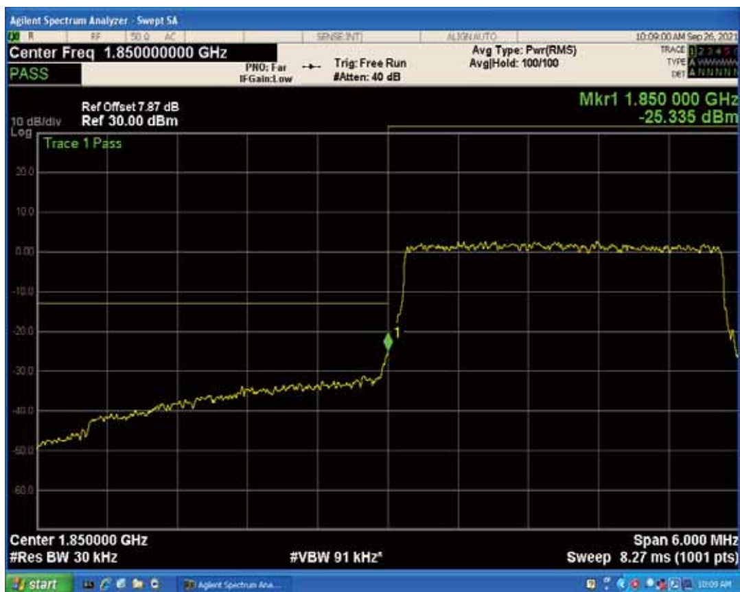
Band2 QAM16 BW=3MHz Channel=18615 RB Size=1 Position=#0
