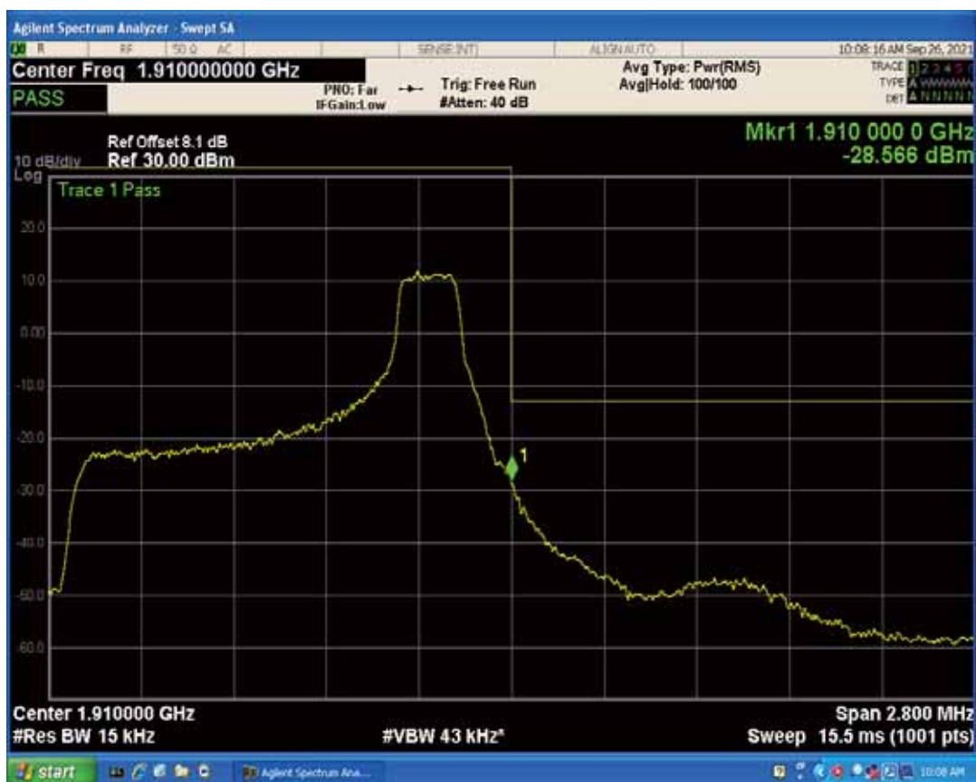
Band2 QPSK BW=1.4MHz Channel=19193 RB Size=6 Position=#0
