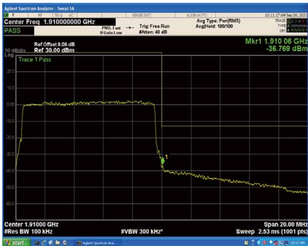
Band2 QAM16 BW=10MHz Channel=19150 RB Size=1 Position=#0
