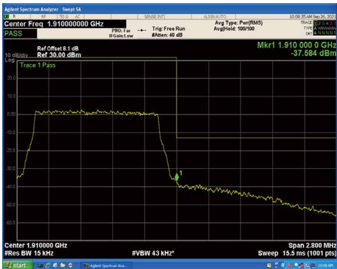
Band2 QPSK BW=3MHz Channel=18615 RB Size=1 Position=#Max
