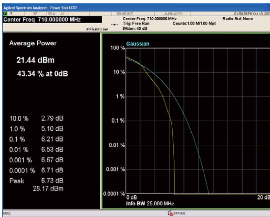
Band17 QAM16 BW=10MHz Channel=23790 RB Size=1 Position=#0
