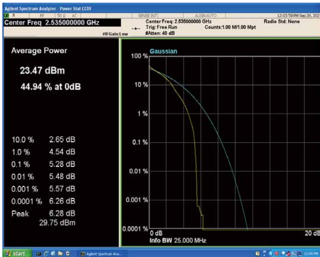
Band7 QAM16 BW=15MHz Channel=21100 RB Size=1 Position=#0
