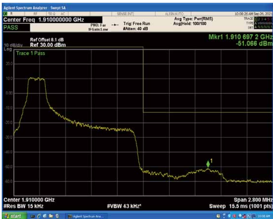
Band2 QAM16 BW=1.4MHz Channel=19193 RB Size=1 Position=#Max
