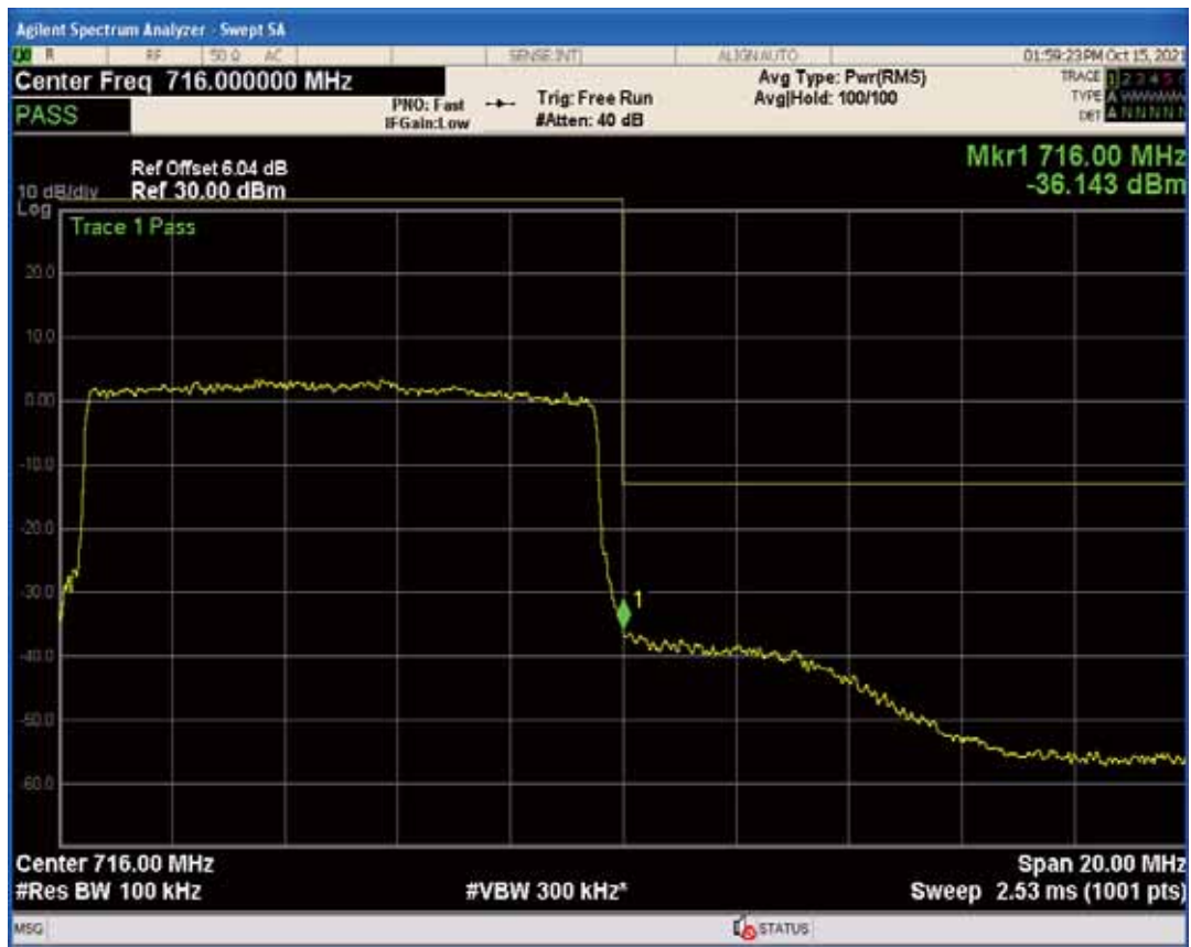
Band2 QPSK BW=1.4MHz Channel=18607 RB Size=1 Position=#Max
