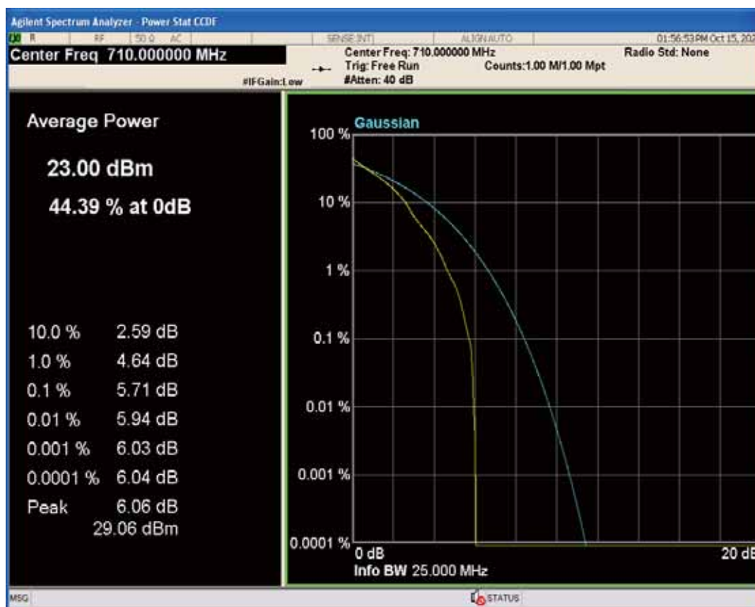
Band17 QAM16 BW=5MHz Channel=23790 RB Size=1 Position=#0
