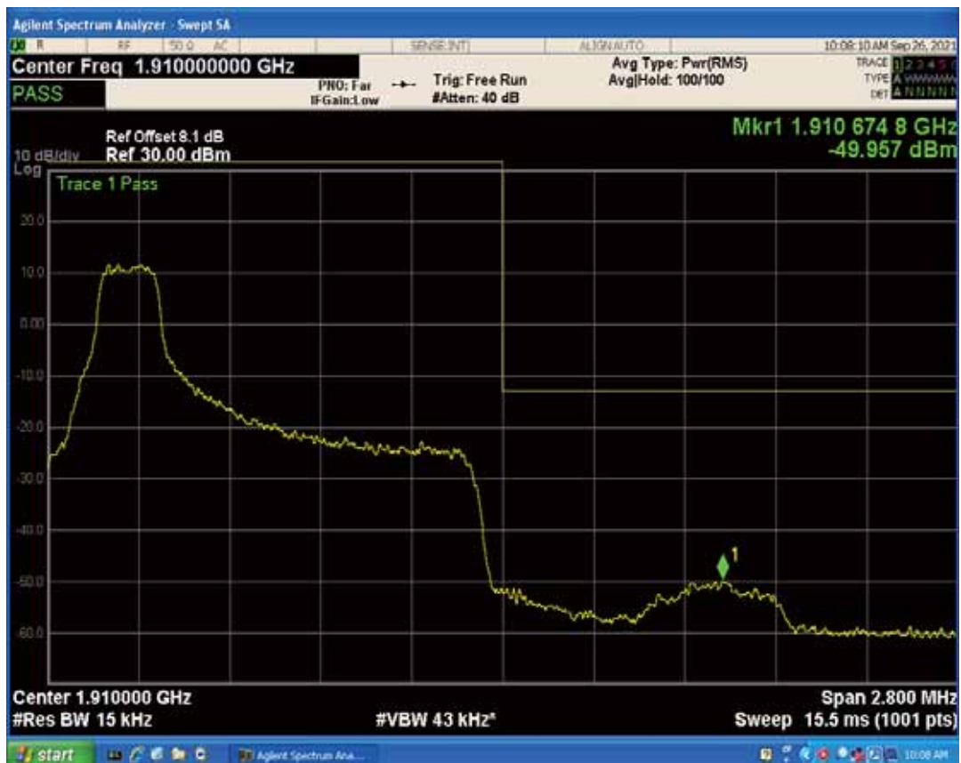
Band2 QPSK BW=1.4MHz Channel=19193 RB Size=1 Position=#Max
