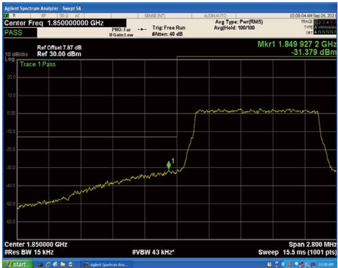
Band2 QPSK BW=1.4MHz Channel=19193 RB Size=1 Position=#0
