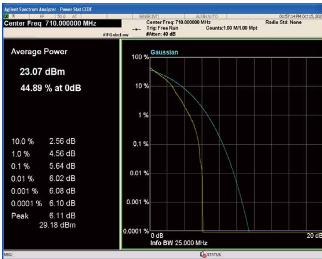
Band2 QPSK BW=1.4MHz Channel=18900 RB Size=1 Position=#0
