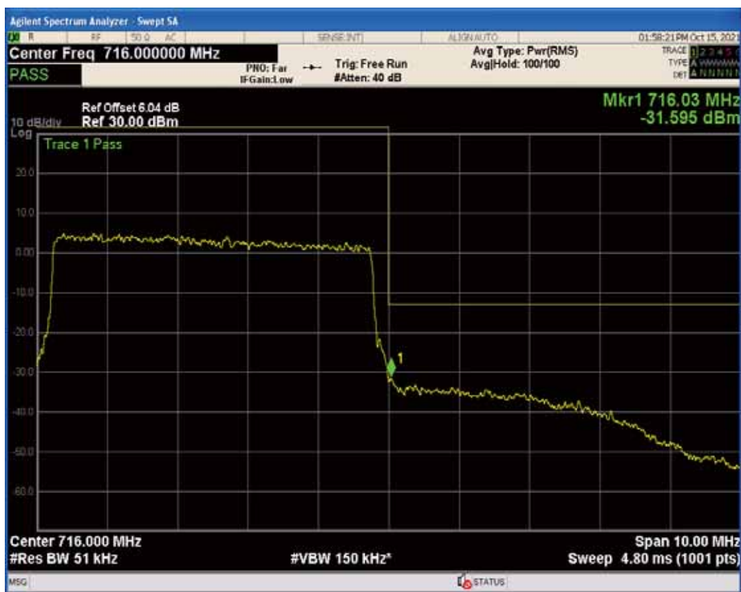
Band17 QAM16 BW=5MHz Channel=23825 RB Size=1 Position=#Max
