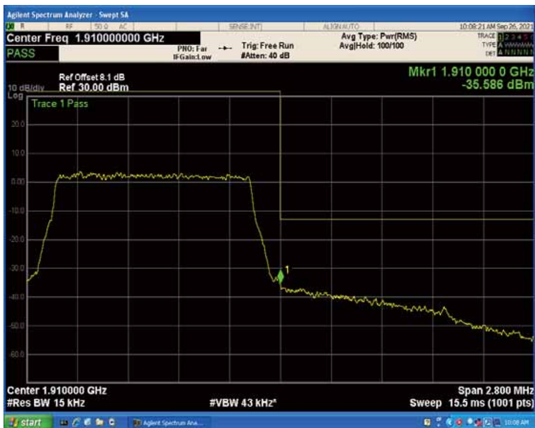
Band2 QAM16 BW=1.4MHz Channel=19193 RB Size=1 Position=#0
