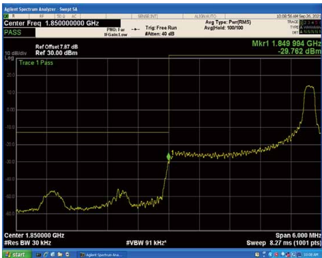
Band2 QPSK BW=3MHz Channel=18615 RB Size=15 Position=#0
