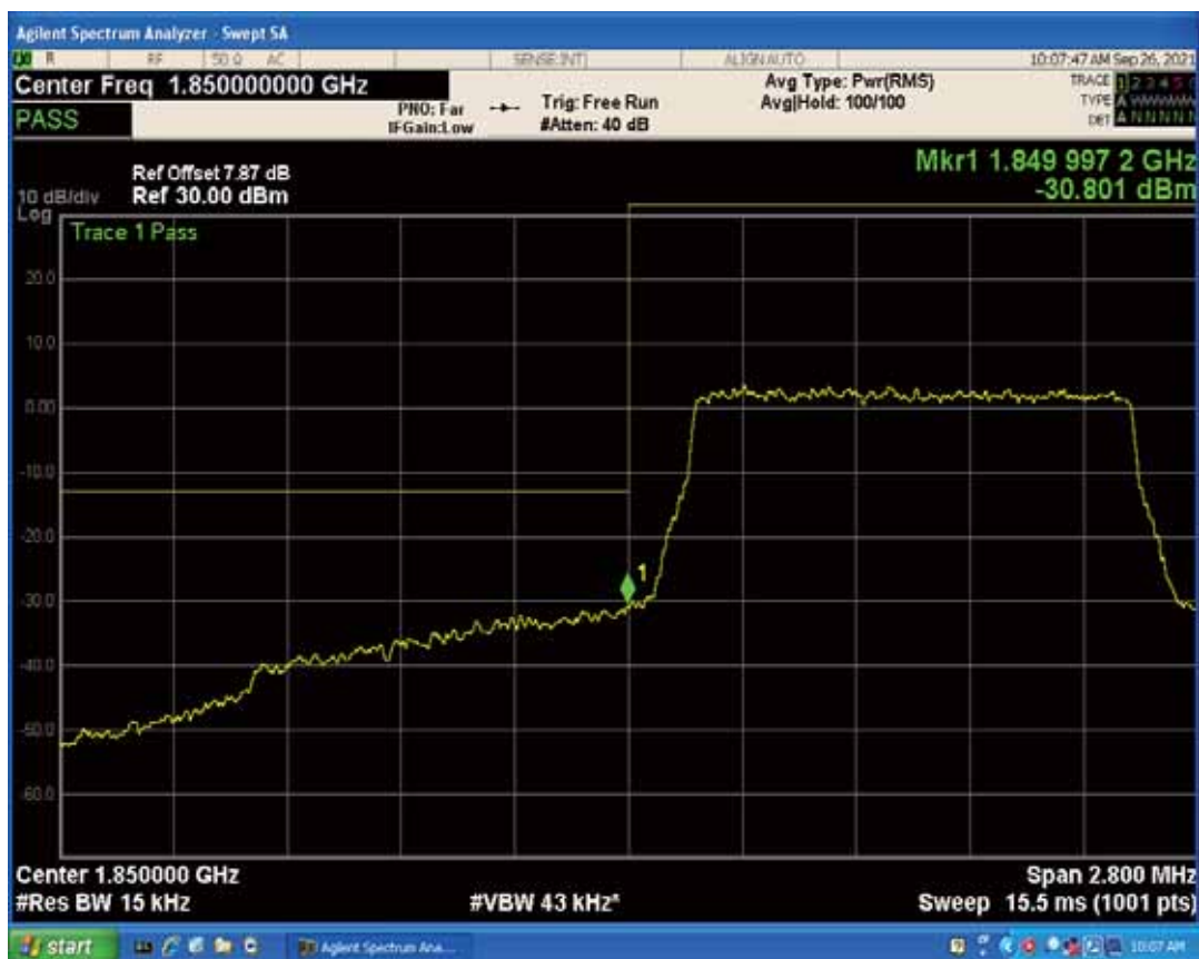
Band2 QAM16 BW=1.4MHz Channel=18607 RB Size=1 Position=#0
