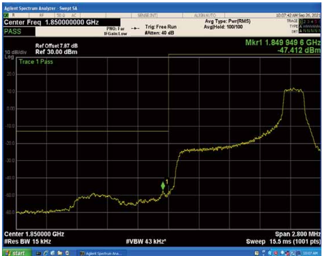
Band2 QPSK BW=1.4MHz Channel=18607 RB Size=1 Position=#0
