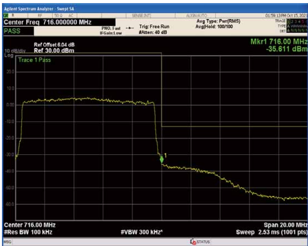
Band17 QPSK BW=10MHz Channel=23800 RB Size=1 Position=#Max
