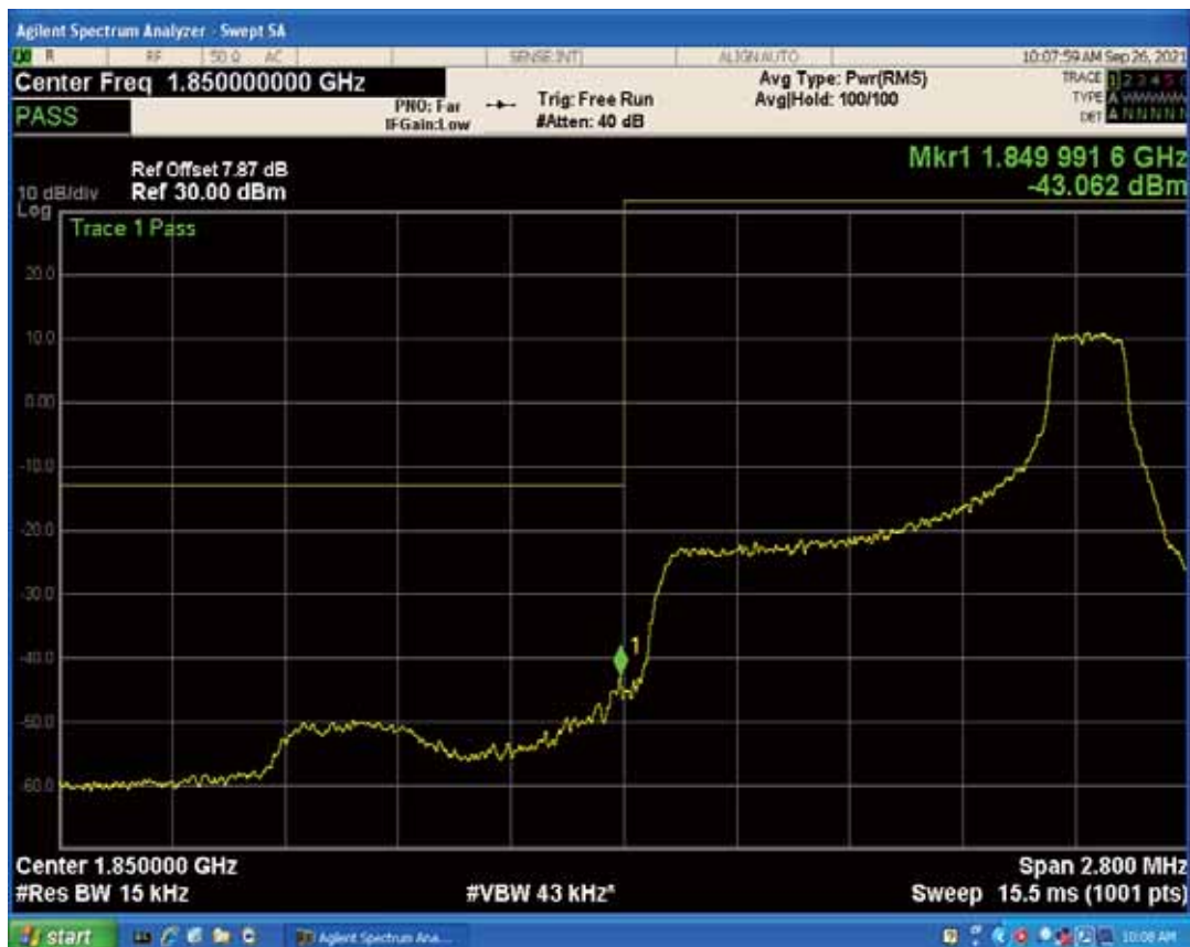
Band2 QAM16 BW=1.4MHz Channel=18607 RB Size=6 Position=#0
