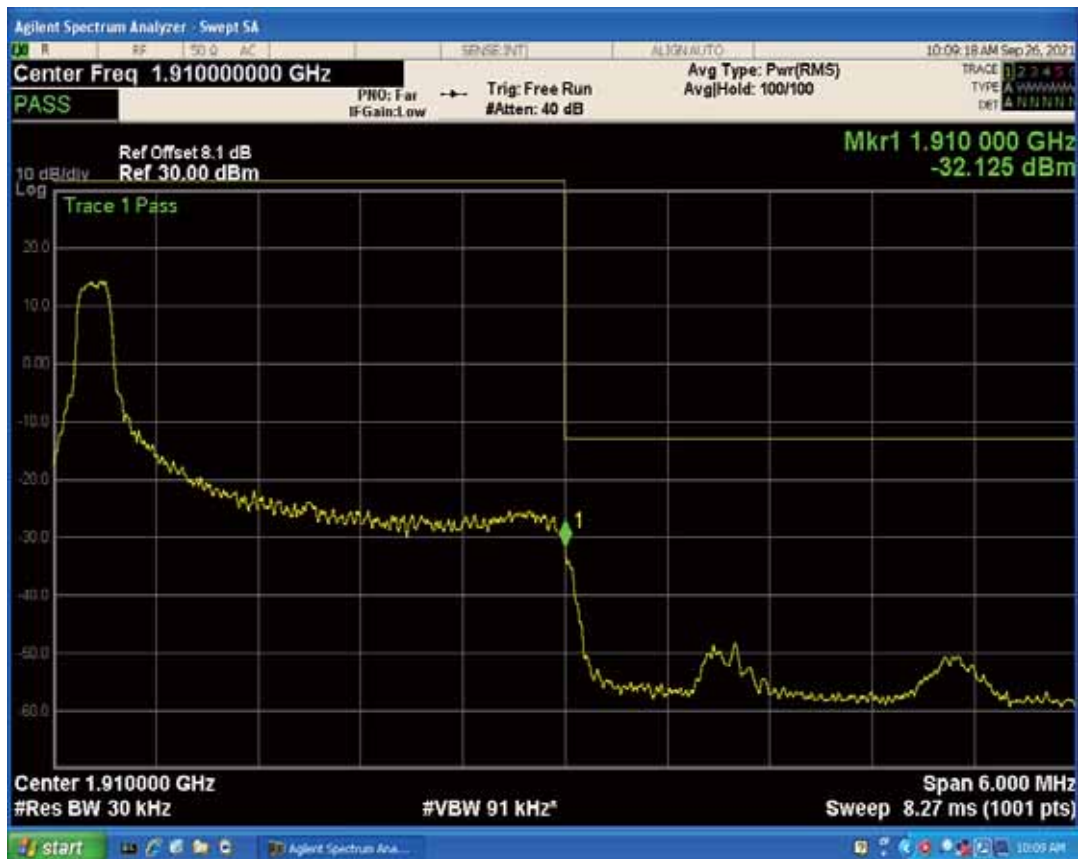
Band2 QPSK BW=3MHz Channel=19185 RB Size=15 Position=#0
