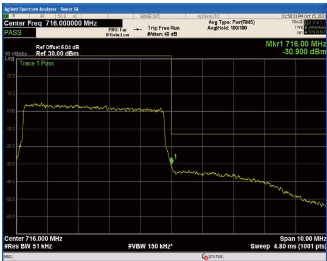
Band17 QPSK BW=10MHz Channel=23780 RB Size=1 Position=#Max
