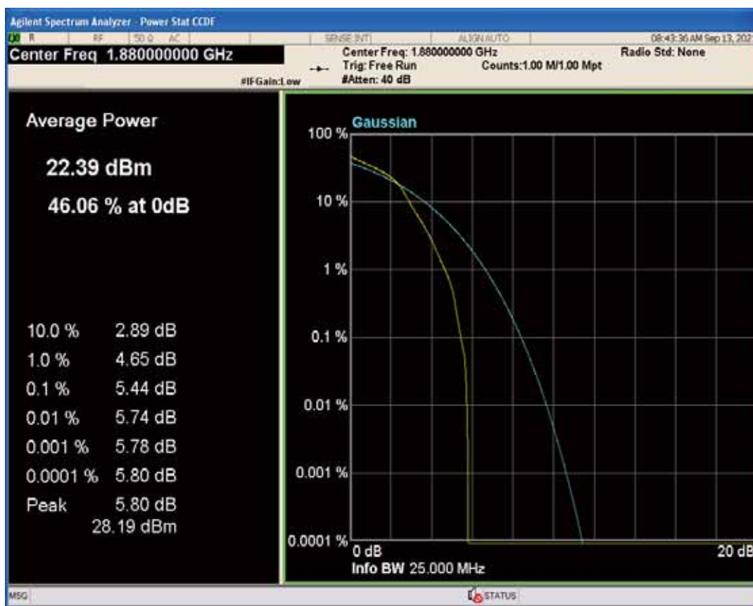
Band2 QAM16 BW=3MHz Channel=18900 RB Size=1 Position=#0
