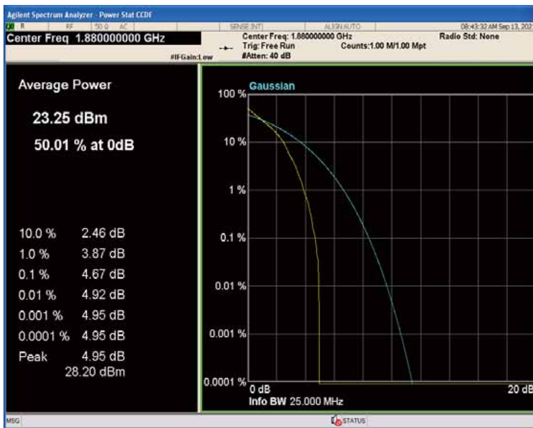
Band2 QAM16 BW=1.4MHz Channel=18900 RB Size=1 Position=#0
