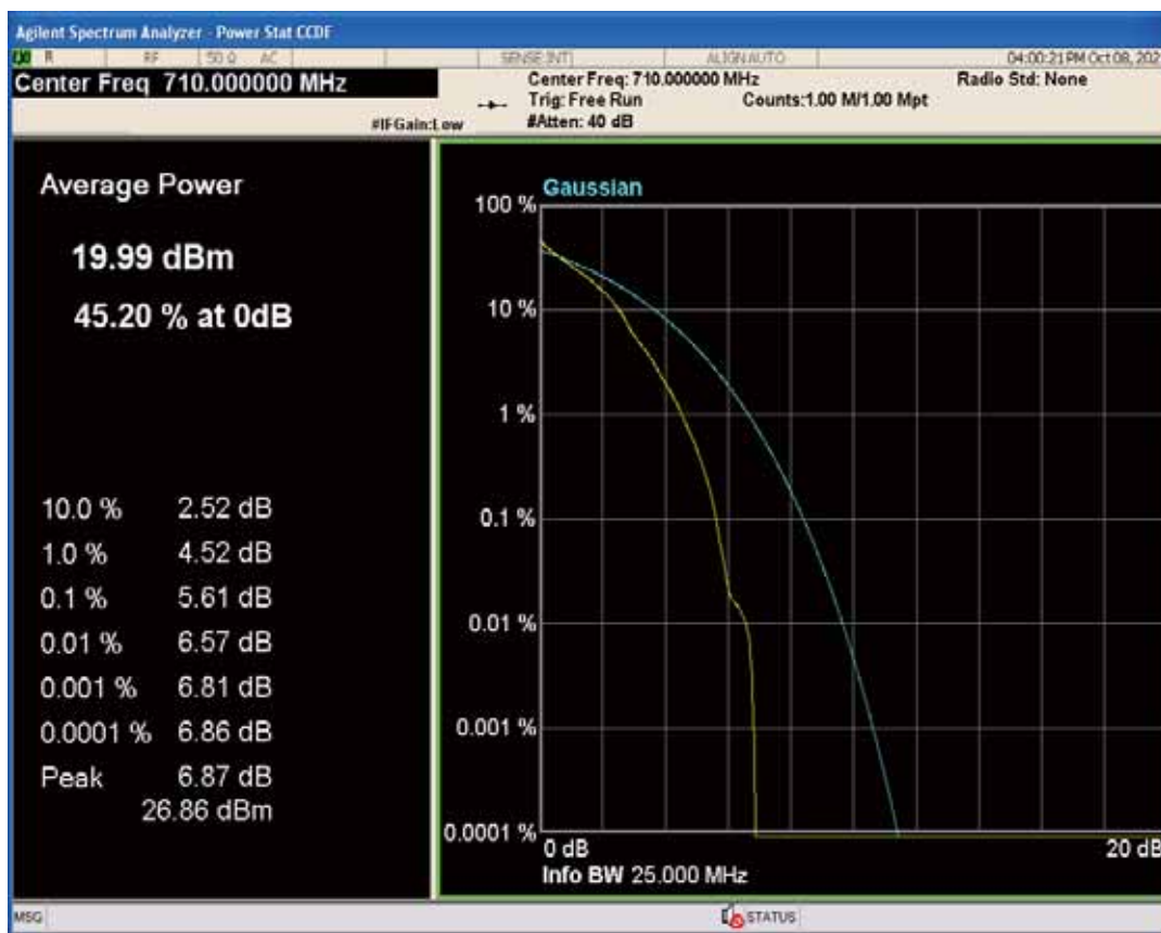
Band17 QAM16 BW=10MHz Channel=23790 RB Size=1 Position=#0
