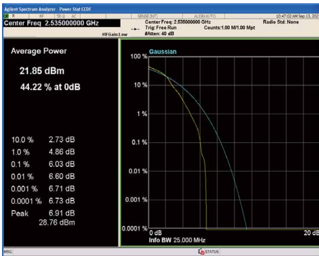
Band7 QPSK BW=15MHz Channel=21100 RB Size=1 Position=#0
