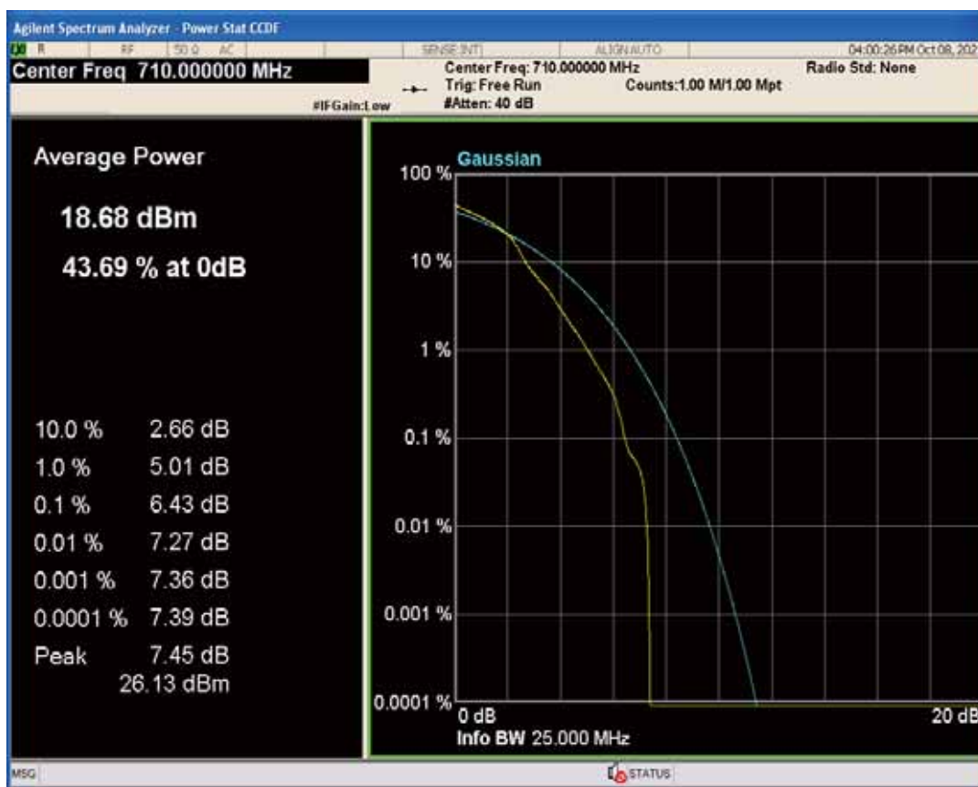
Band2 QPSK BW=1.4MHz Channel=18900 RB Size=1 Position=#0
