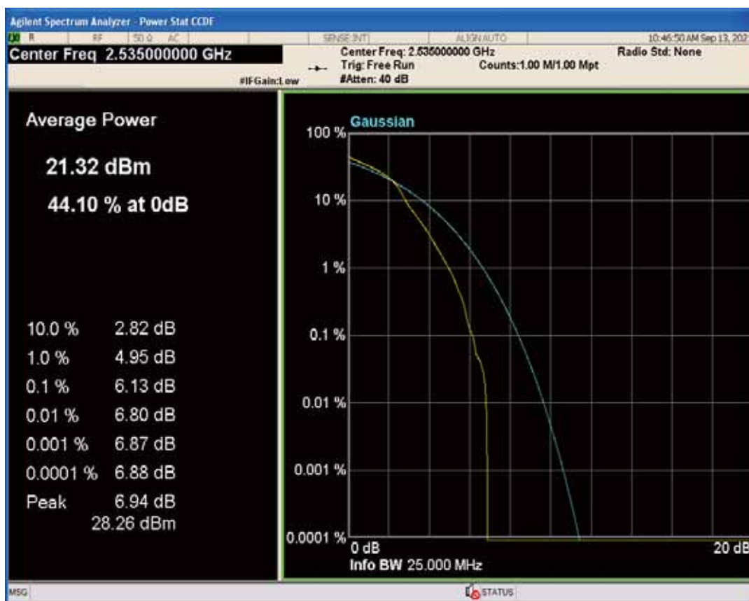
Band7 QPSK BW=10MHz Channel=21100 RB Size=1 Position=#0
