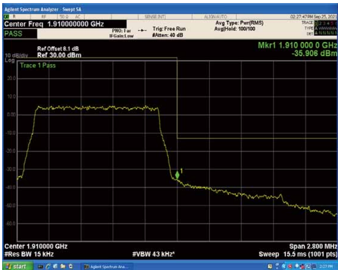
Band2 QPSK BW=1.4MHz Channel=19193 RB Size=1 Position=#Max
