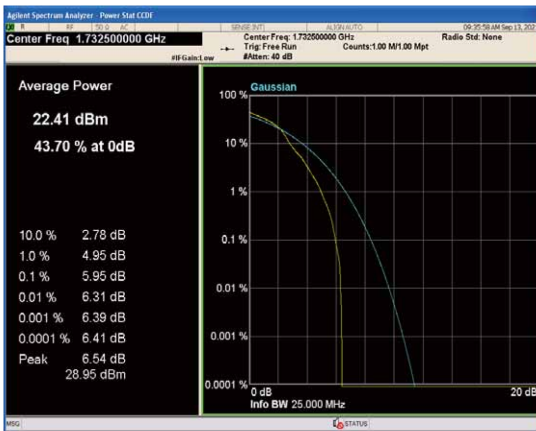
Band4 QPSK BW=15MHz Channel=20175 RB Size=1 Position=#0
