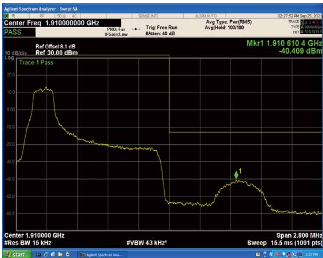
Band2 QAM16 BW=1.4MHz Channel=18607 RB Size=1 Position=#0
