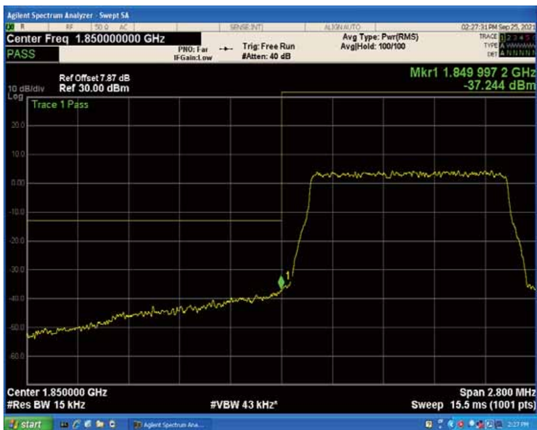
Band2 QAM16 BW=1.4MHz Channel=19193 RB Size=1 Position=#0
