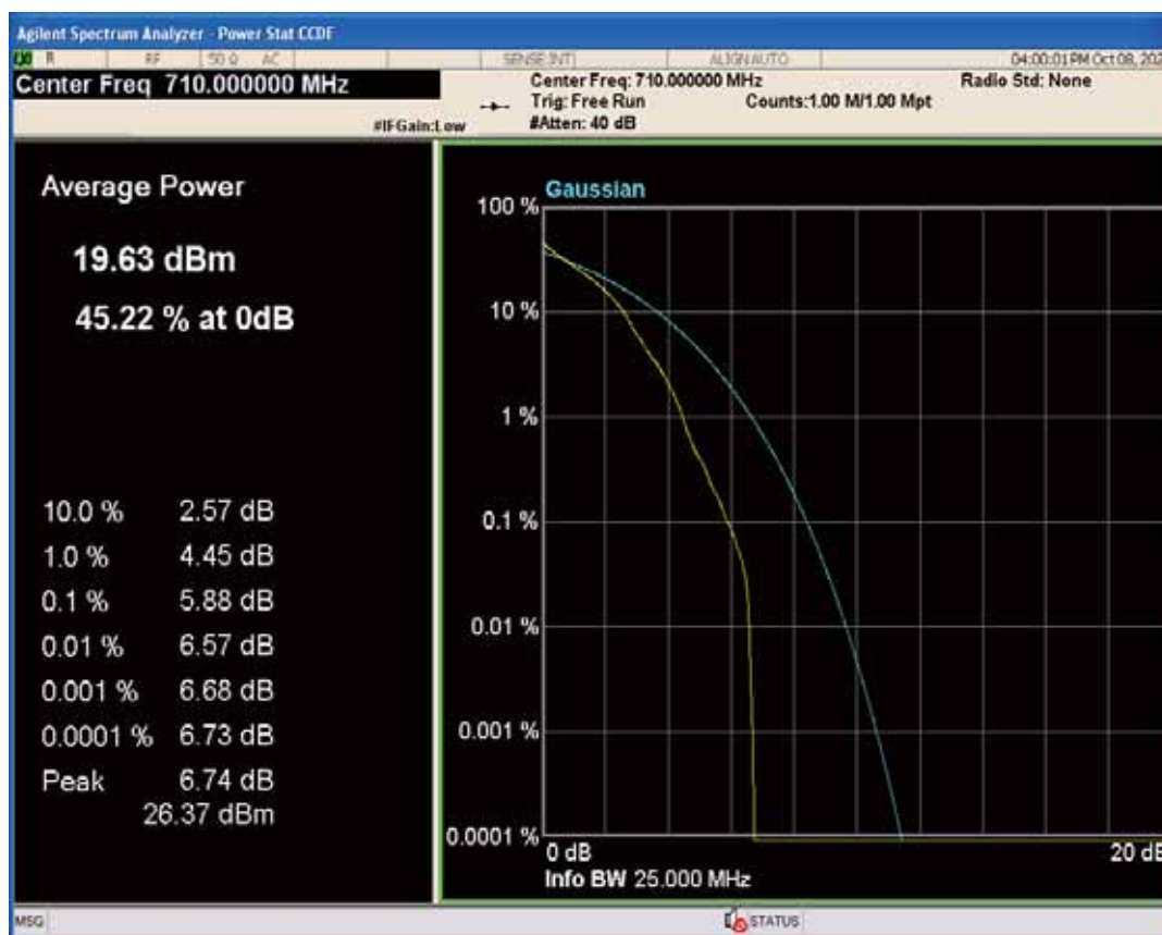
Band17 QAM16 BW=5MHz Channel=23790 RB Size=1 Position=#0
