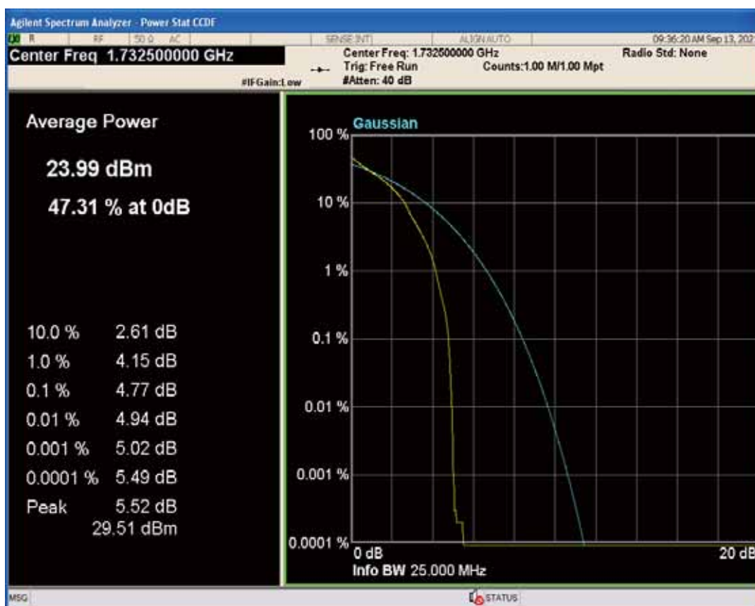
Band4 QAM16 BW=20MHz Channel=20175 RB Size=1 Position=#0
