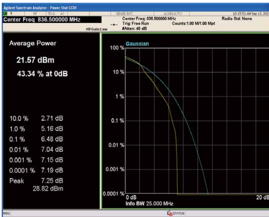
Band7 QPSK BW=5MHz Channel=21100 RB Size=1 Position=#0
