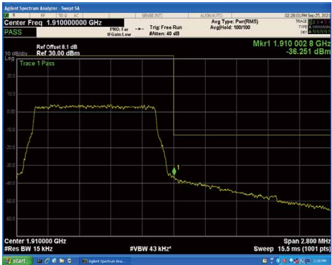
Band2 QAM16 BW=1.4MHz Channel=19193 RB Size=1 Position=#Max
