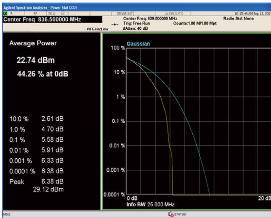
Band5 QAM16 BW=10MHz Channel=20525 RB Size=1 Position=#0
