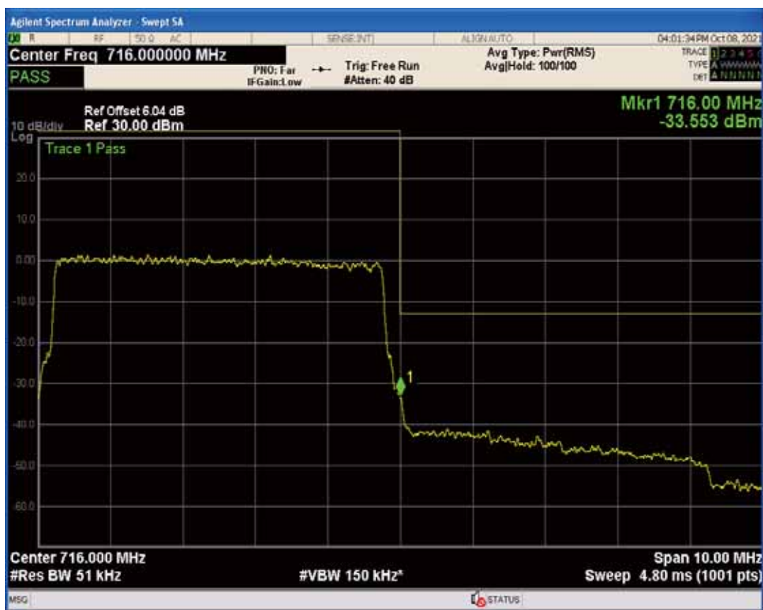
Band17 QAM16 BW=5MHz Channel=23825 RB Size=1 Position=#Max
