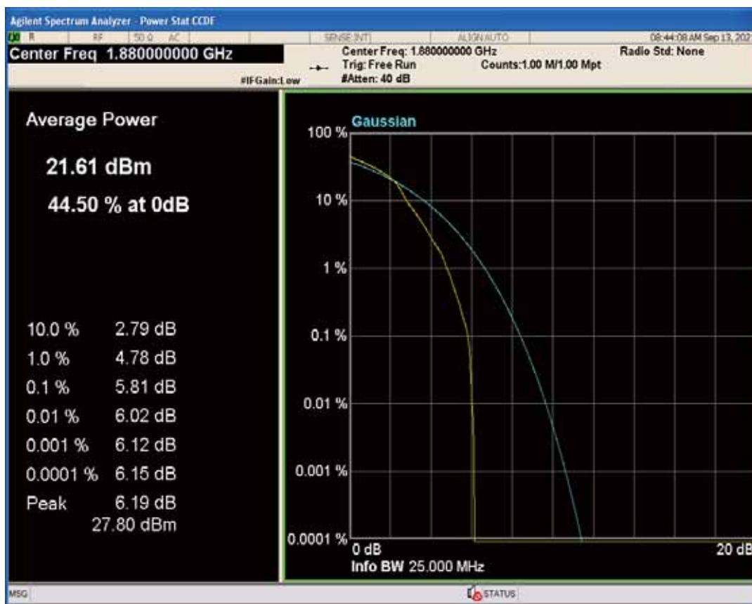
Band2 QAM16 BW=10MHz Channel=18900 RB Size=1 Position=#0
