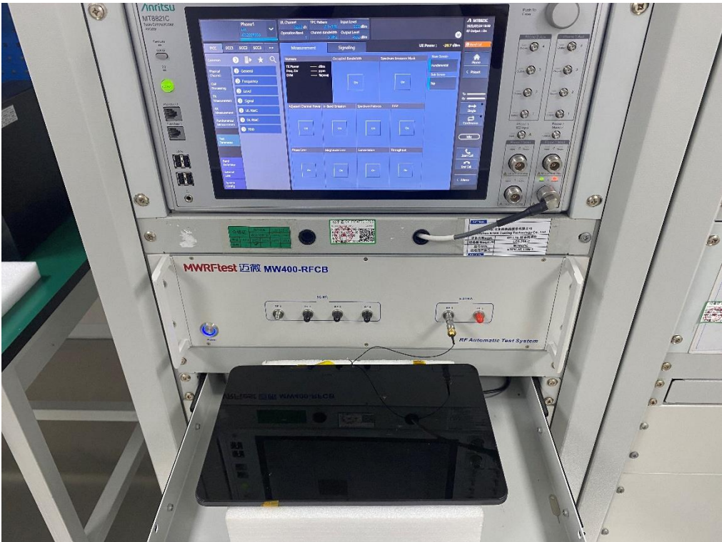
RF Conducted Measurement Photos
