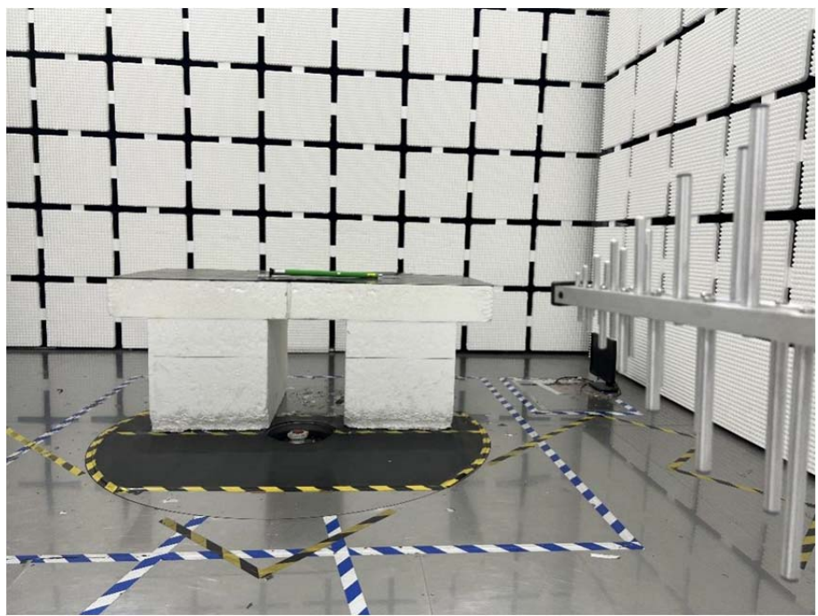
Radiation Emission Test Setup (30MHz to 1GHz)
