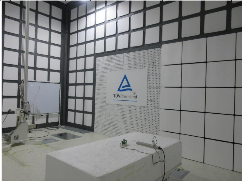
Photograph 8: Test Setup for Spurious Emissions (Back View 2, 5Vdc)
