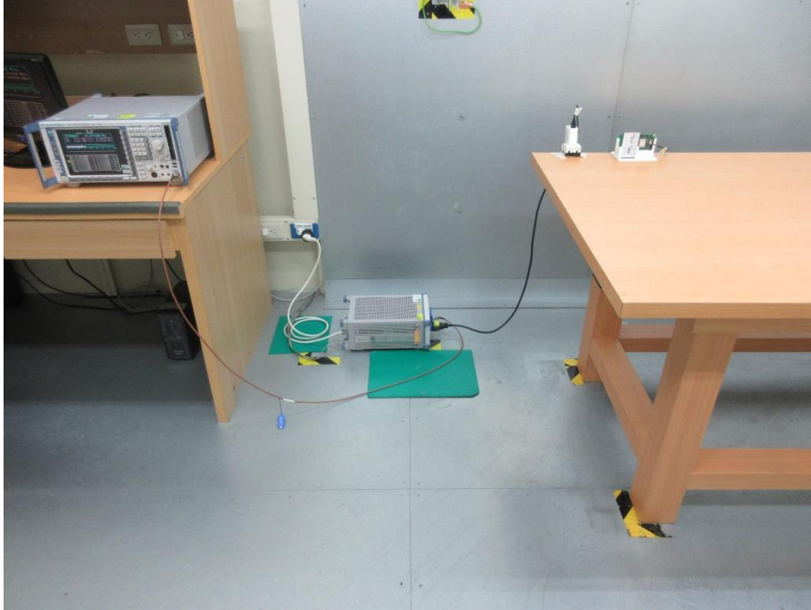
Photograph 9: Test Setup for Mains Conducted Emissions (Front View, 5Vdc)
