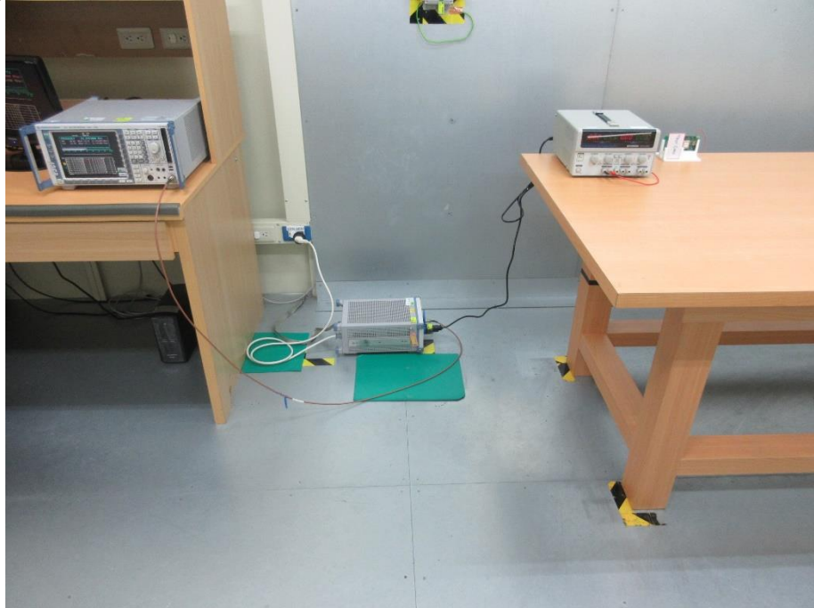
Photograph 4: Test Setup for Mains Conducted Emissions (Front View, 3.3Vdc)
