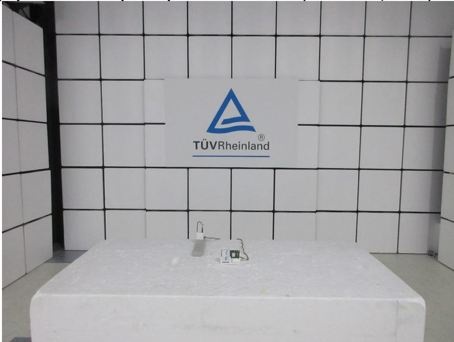
Photograph 6: Test Setup for Spurious Emissions (Front View, 5 Vdc)
