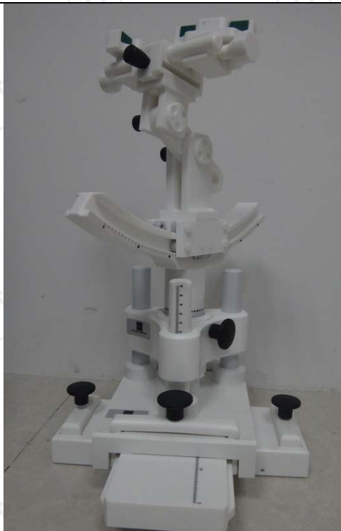
COMOSAR Mobile phone positioning system
