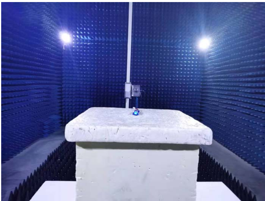
Photo of Radiated Emission Measurement Above 1GHz
