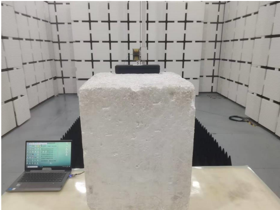
Set-up for Radiated Spurious Emission, Above 1GHz
