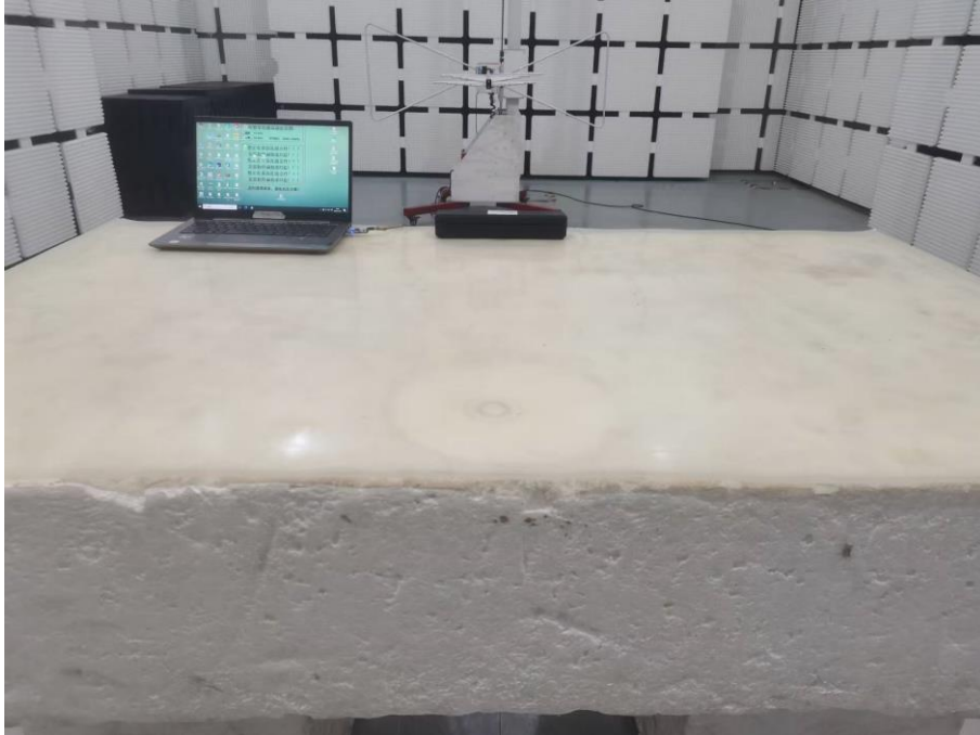
Set-up for Radiated Spurious Emission, Above 1GHz
