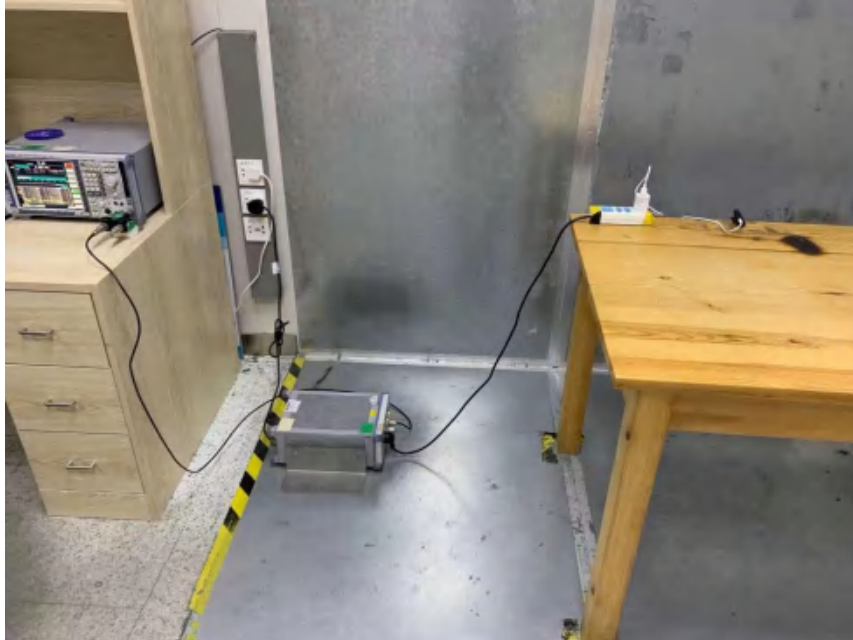
Radiated Spurious Emissions From 30M-1GHz
