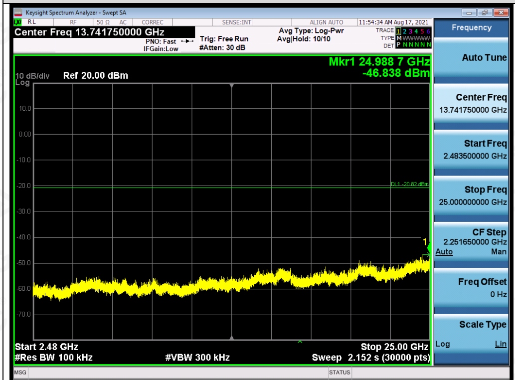
Test_Graph_802.11n40_ANT1_2437_MCS0_Higher Band Emissions
