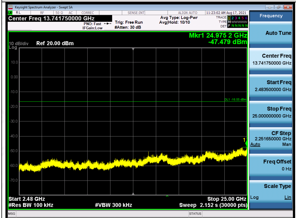
Test_Graph_802.11n20_ANT1_2437_MCS0_Higher Band Emissions
