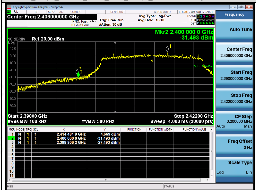
Test_Graph_802.11g_ANT1_2412_6Mbps_Lower Band Edge Emissions
