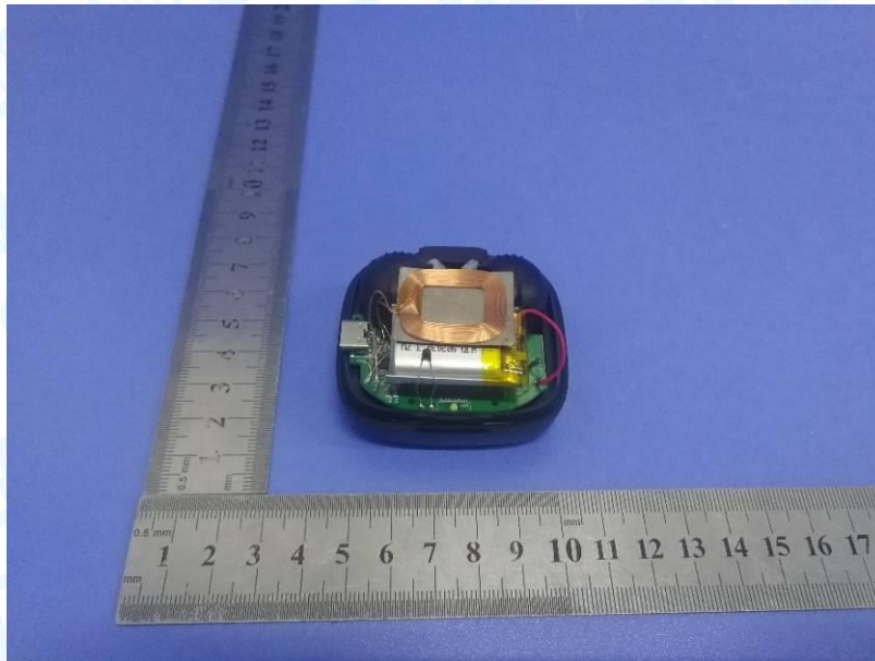
Photo 14 Appearance of Battery
