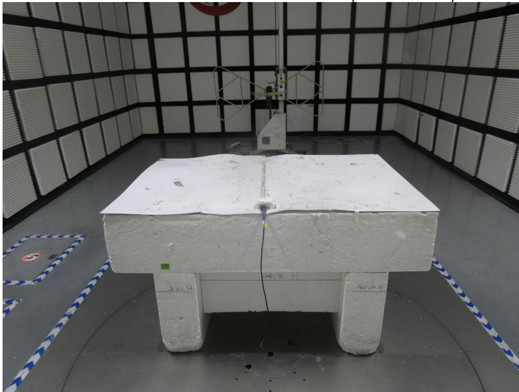
RADIATED RF MEASUREMENT SETUP (Below 30MHz)
