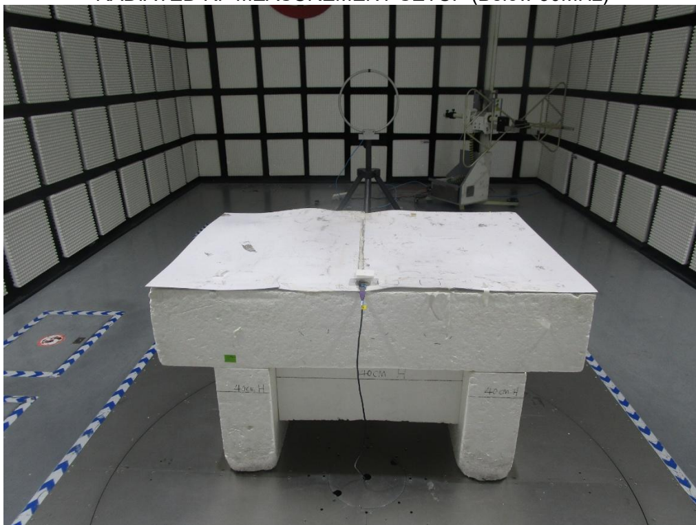
RADIATED RF MEASUREMENT SETUP (Below 30MHz)
