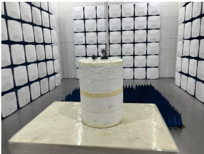
Radiated Emission (18GHz-25GHz)
