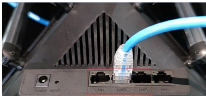
Router connect network cable
