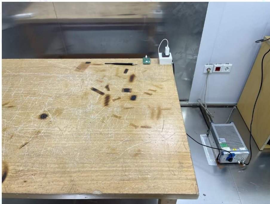
Photo of Setup for Radiated Emission (30MHz~1GHz)
