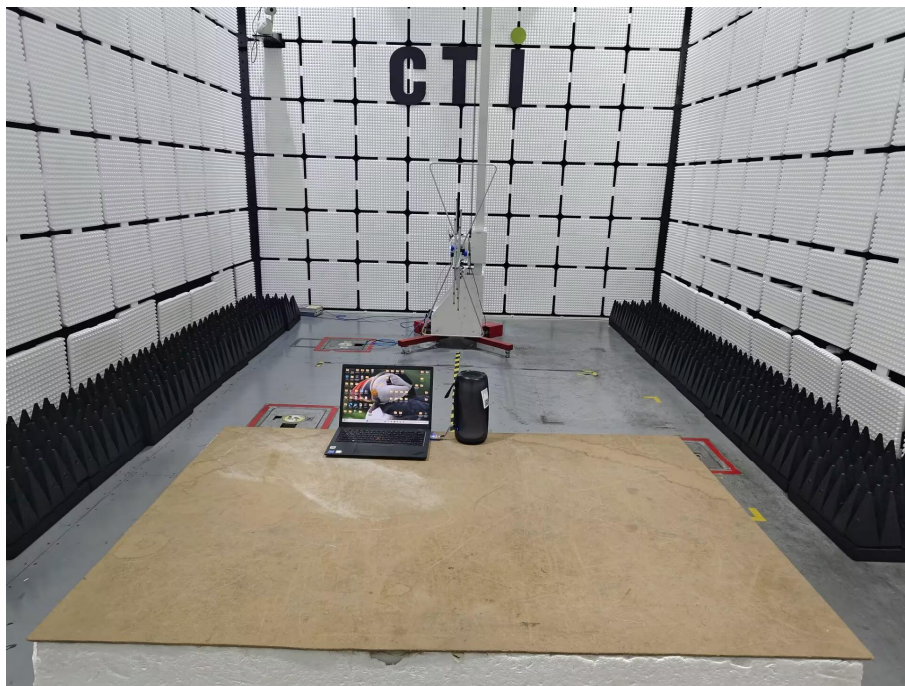
Radiated spurious emission Test Setup-1(Below 1GHz)
