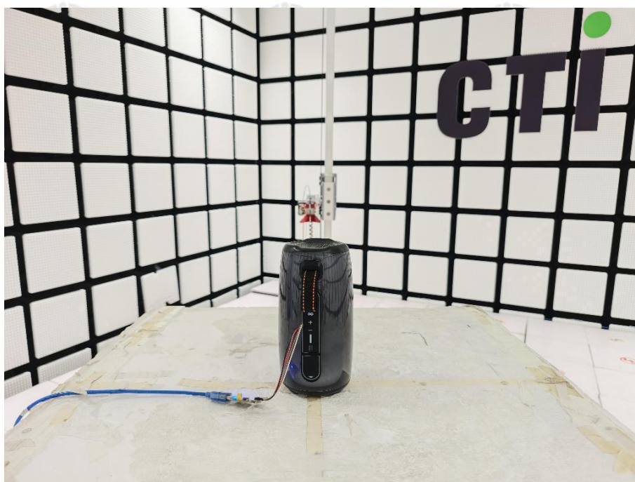
Radiated spurious emission Test Setup-2(Above 1GHz)
