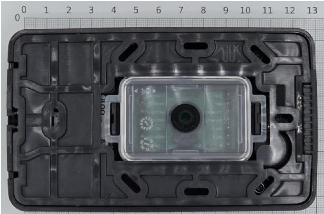
Figure 6: N510.200, Bottom view. Mounting bracket assembled.
