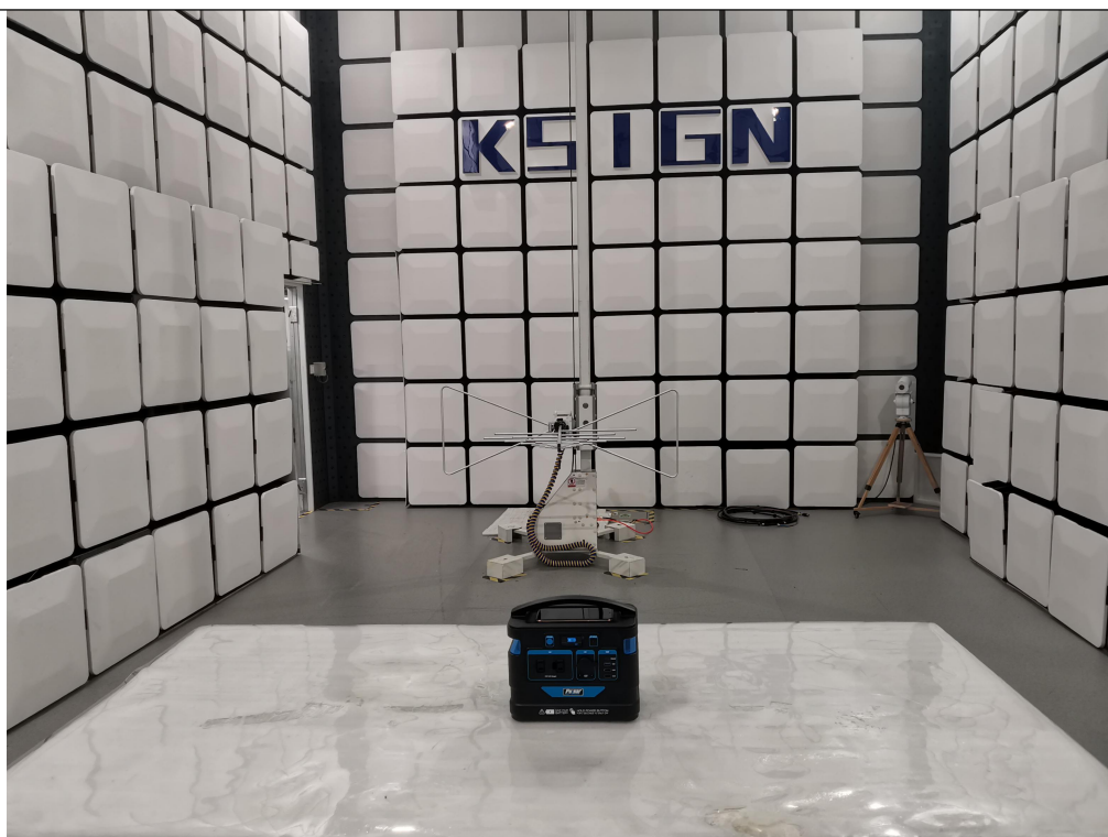
RADIATED EMISSION TEST SETUP(30MHz-1GHz)
