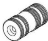
Back damper and decompression cylinder
