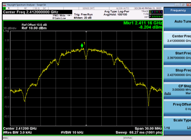
Power spectral density-802.11b ,2462MHz,Ant0
