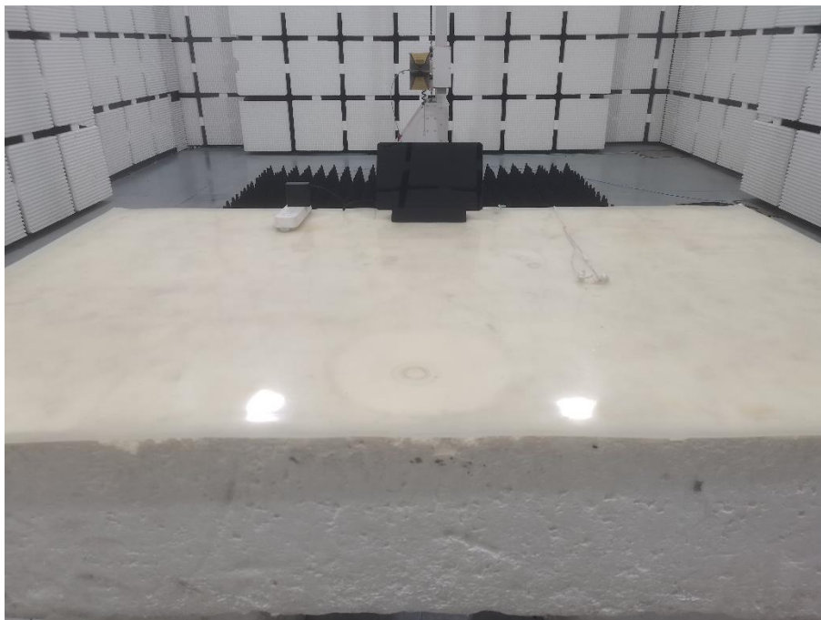
Set-up for Radiated Spurious Emission, Above 1GHz
