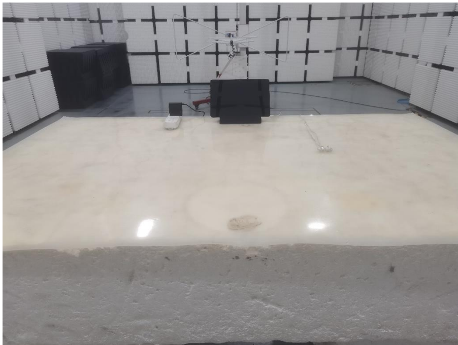
Set-up for Radiated Spurious Emission, Above 1GHz
