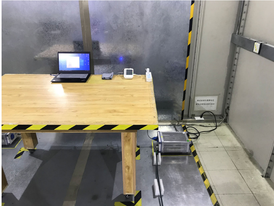
Conducted Emissions (Left View)
