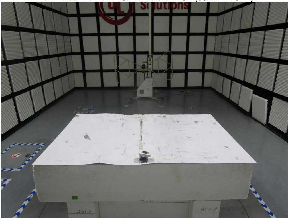
RADIATED RF MEASUREMENT SETUP (Below 30MHz)
