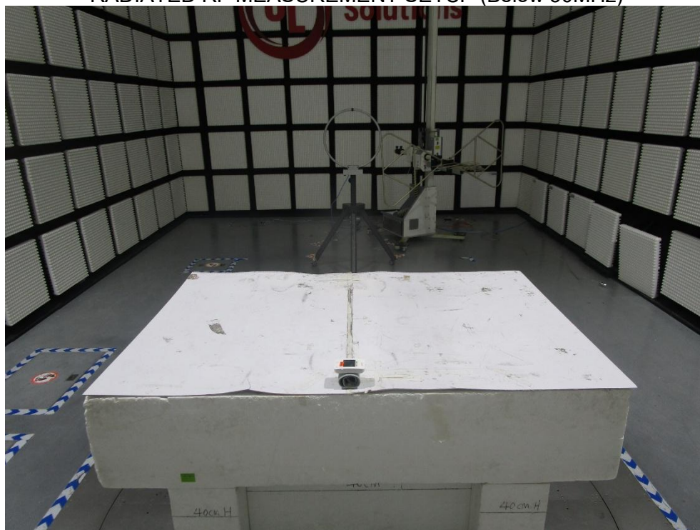
RADIATED RF MEASUREMENT SETUP (Below 30MHz)
