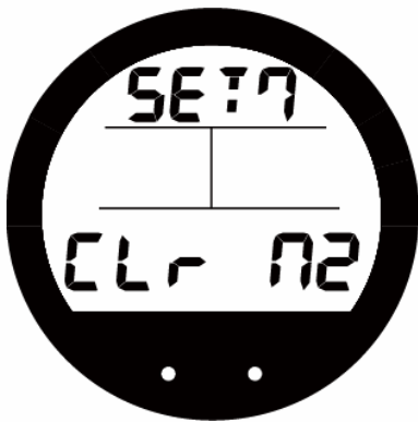
Set Screen - Set7 - Clear residual nitrogen calculation
