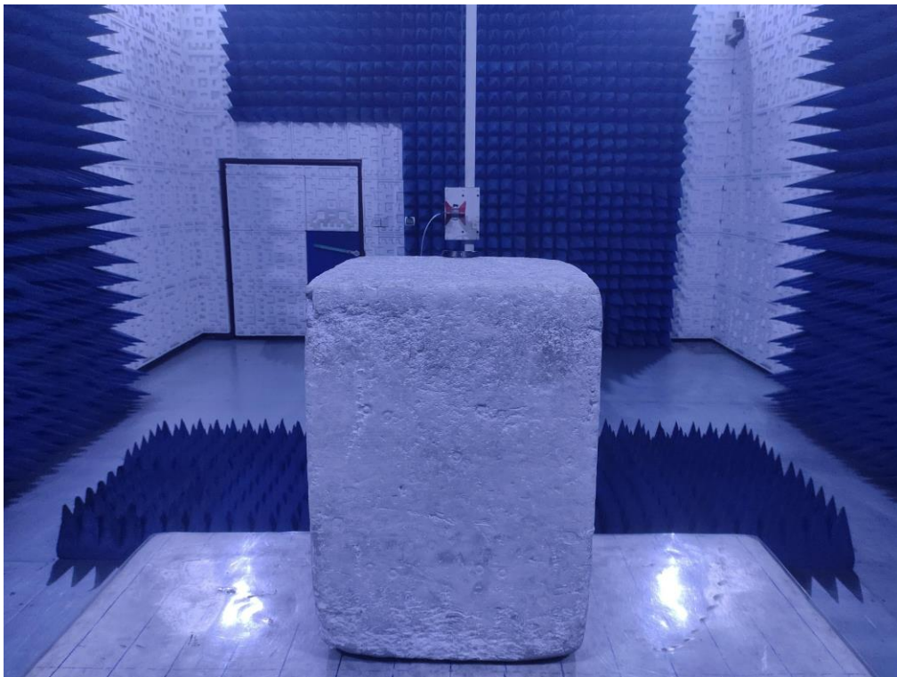
RADIATED EMISSION TEST SETUP ABOVE 1GHz
