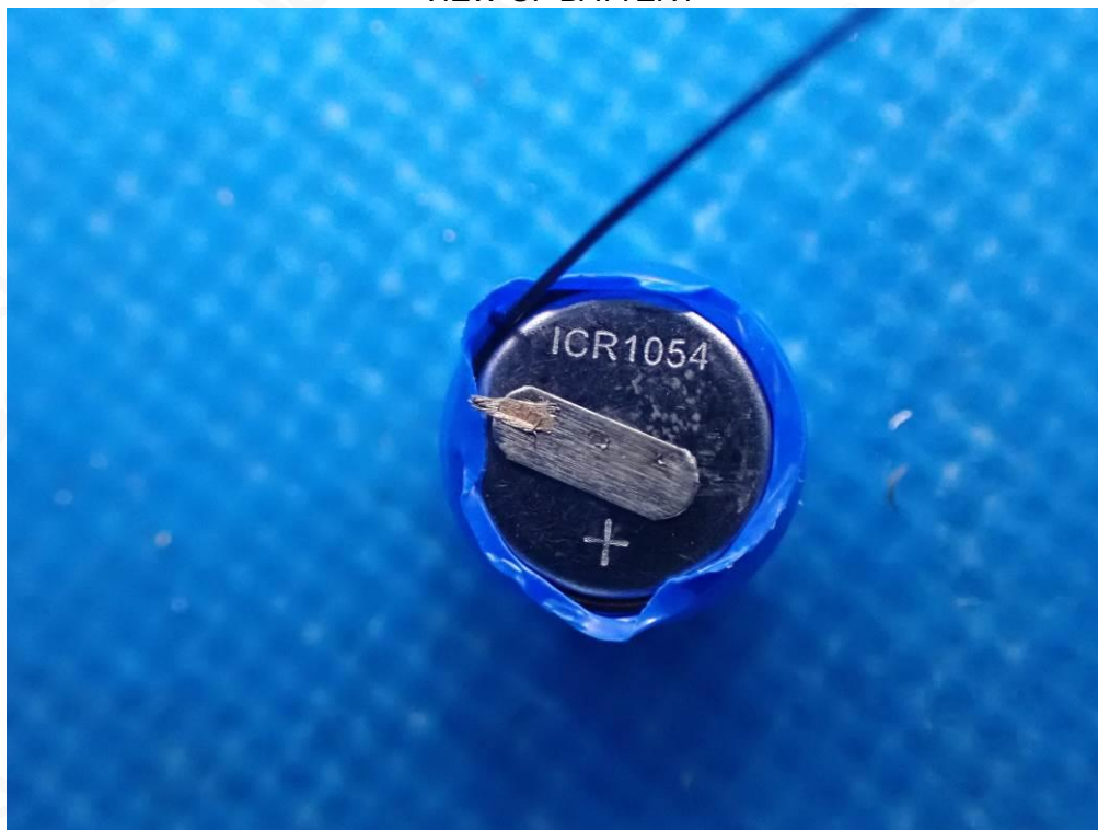
VIEW OF BATTERY
