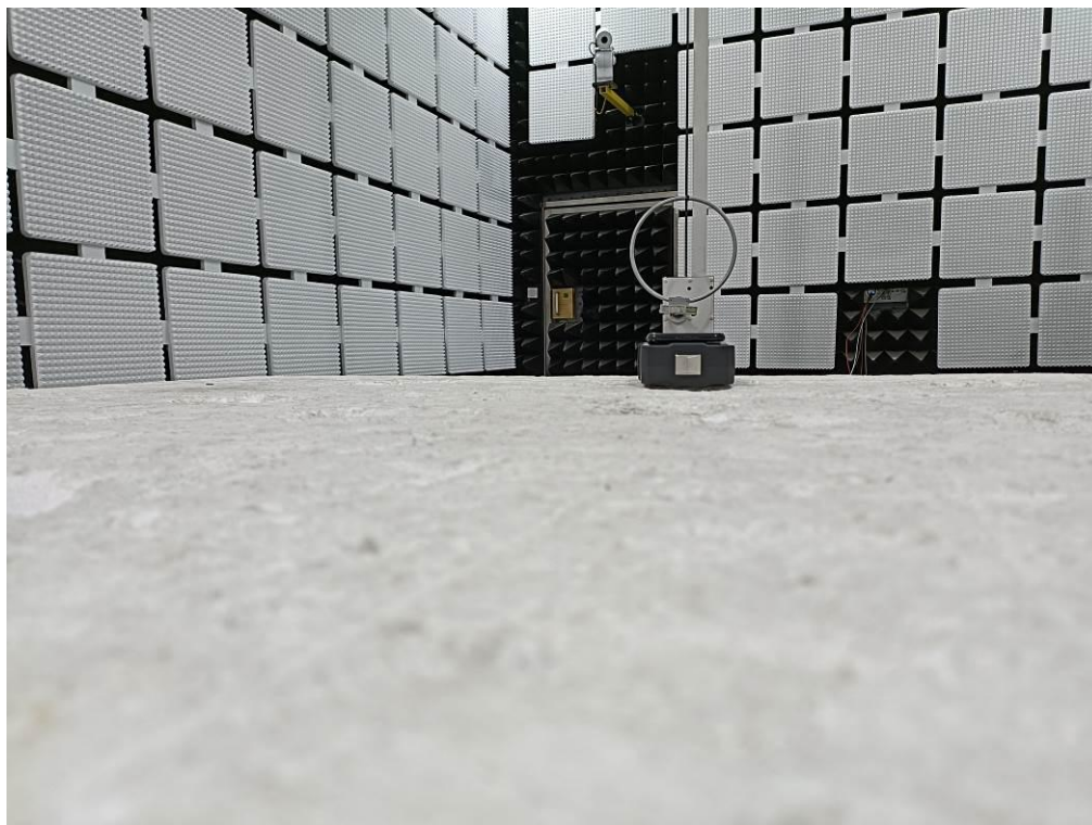
Radiated Emission below 30MHz-AC adapter charge mode
