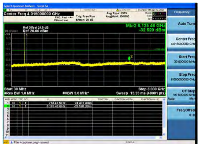
Band12 / 3MHz / High CH / 16QAM
