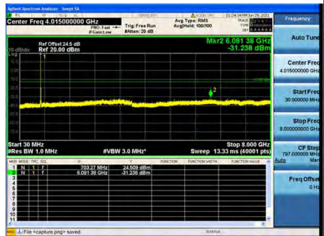
Band12 / 10MHz / High CH / 16QAM
