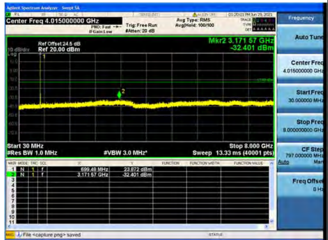
Band12 / 3MHz / Mid CH / 16QAM
