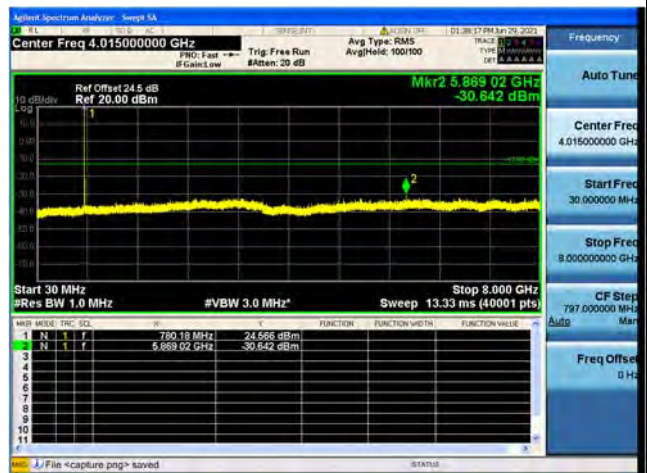
Band13 / 5MHz / High CH / 16QAM
