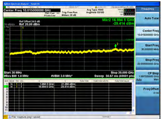
Band25 / 1.4MHz / Mid CH / 16QAM
