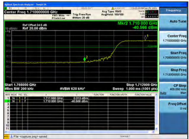
Band4 / 20MHz / High CH / QPSK / FULL RB
