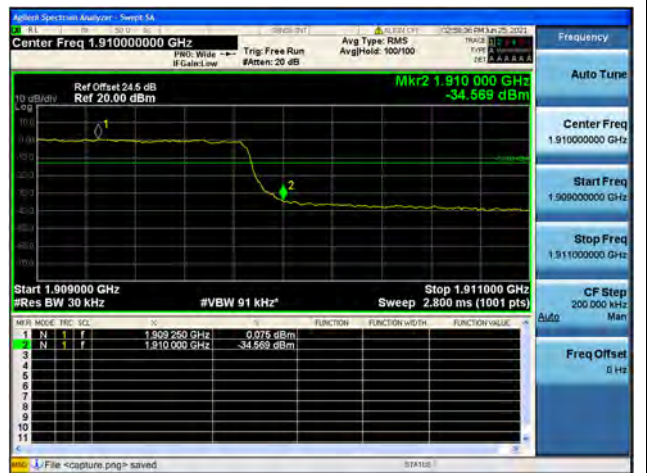
Band2 / 3MHz / High CH / QPSK / FULL RB
