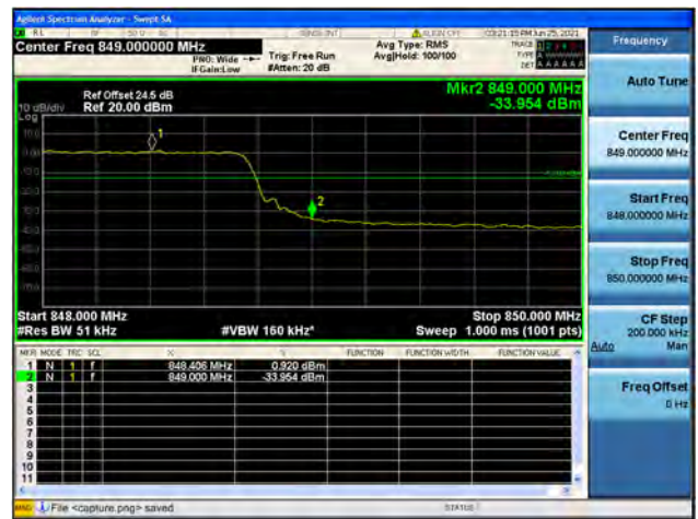
Band5 / 5MHz / High CH / QPSK / FULL RB
