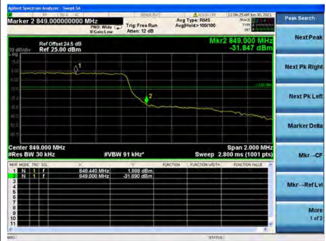
Band26 / 1.4MHz / High CH / QPSK / FULL RB
