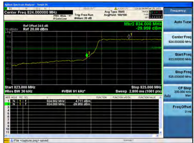
Band5 / 1.4MHz / High CH / QPSK / FULL RB
