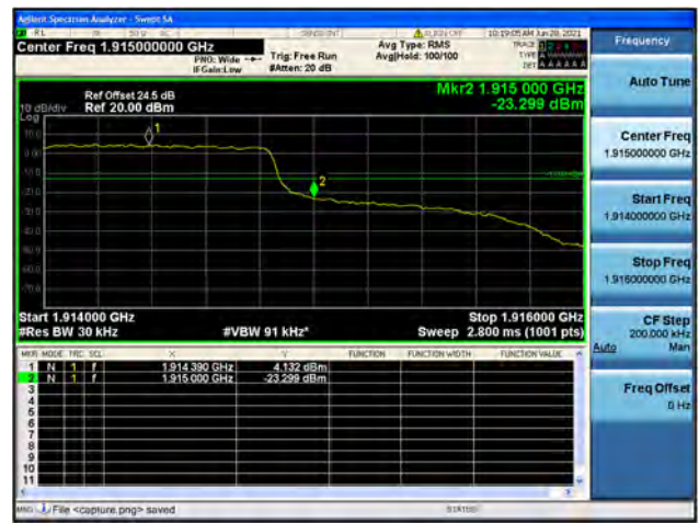
Band25 / 1.4MHz / High CH / QPSK / FULL RB
