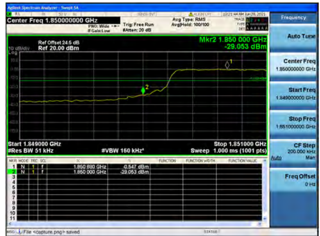
Band25 / 5MHz / High CH / QPSK / FULL RB
