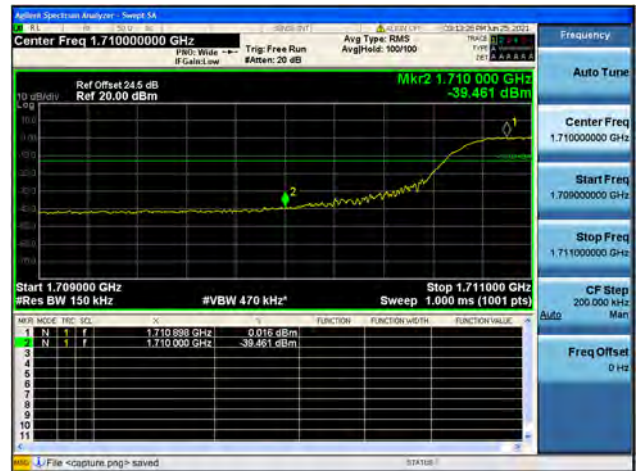
Band4 / 15MHz / High CH / QPSK / FULL RB
