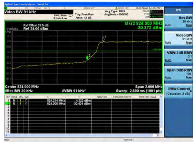
Band26 / 1.4MHz / High CH / QPSK / FULL RB
