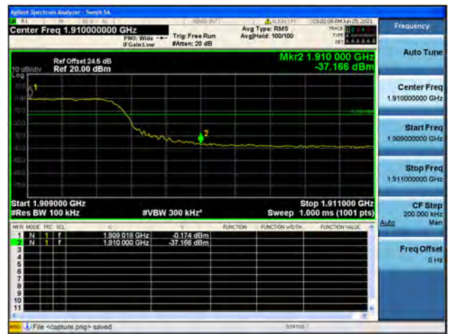
Band2 / 10MHz / High CH / QPSK / FULL RB
