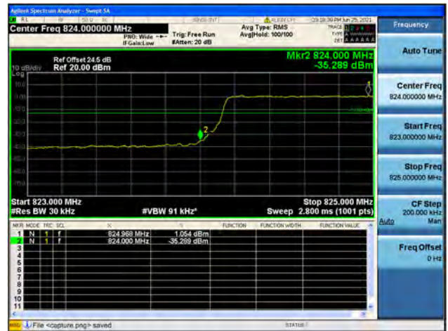
Band5 / 3MHz / High CH / QPSK / FULL RB
