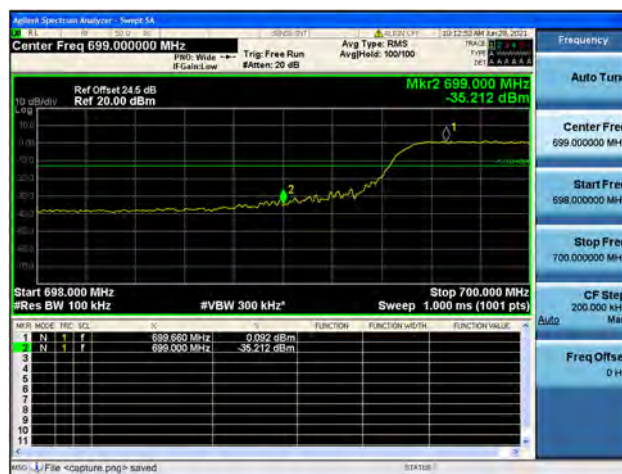
Band12 / 10MHz / High CH / QPSK / FULL RB
