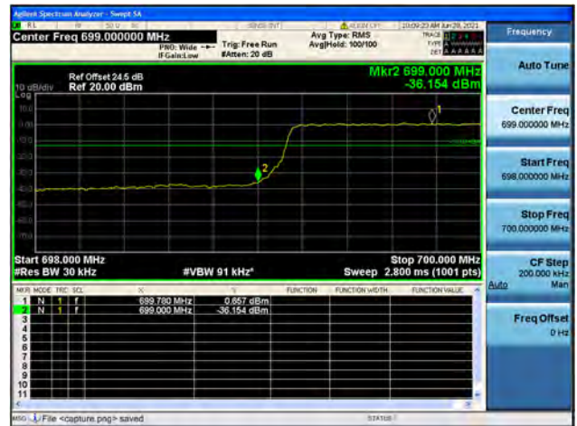
Band12 / 3MHz / High CH / QPSK / FULL RB
