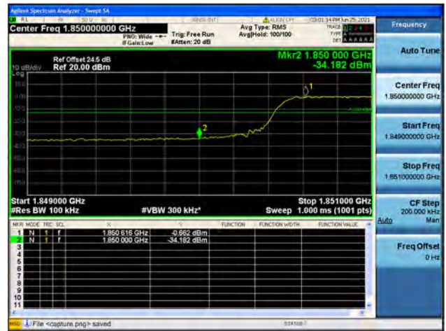
Band2 / 10MHz / High CH / QPSK / FULL RB
