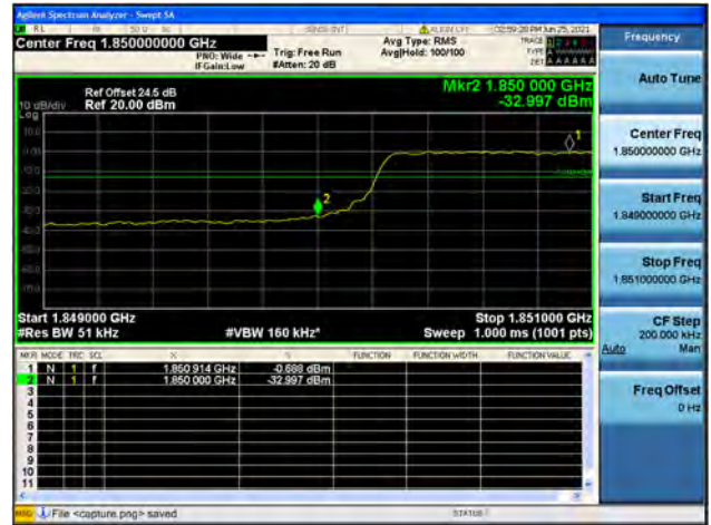
Band2 / 5MHz / High CH / QPSK / FULL RB
