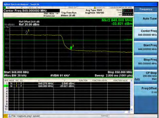
Band5 / 3MHz / High CH / QPSK / FULL RB
