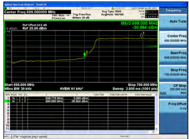
Band12 / 1.4MHz / High CH / QPSK / FULL RB
