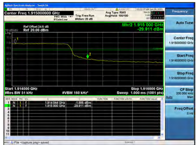
Band25 / 5MHz / High CH / QPSK / FULL RB
