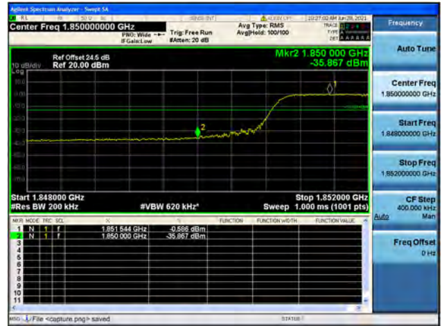
Band25 / 20MHz / High CH / QPSK / FULL RB
