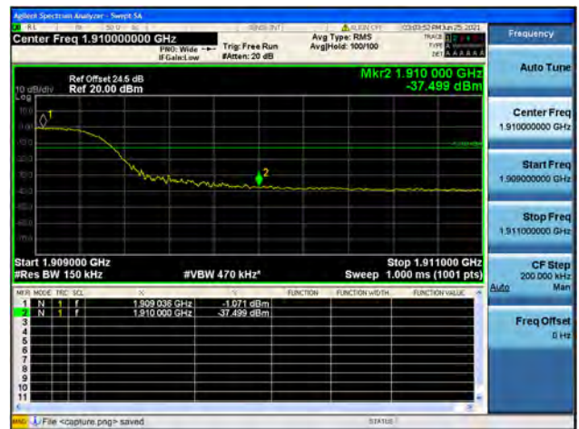
Band2 / 15MHz / High CH / QPSK / FULL RB
