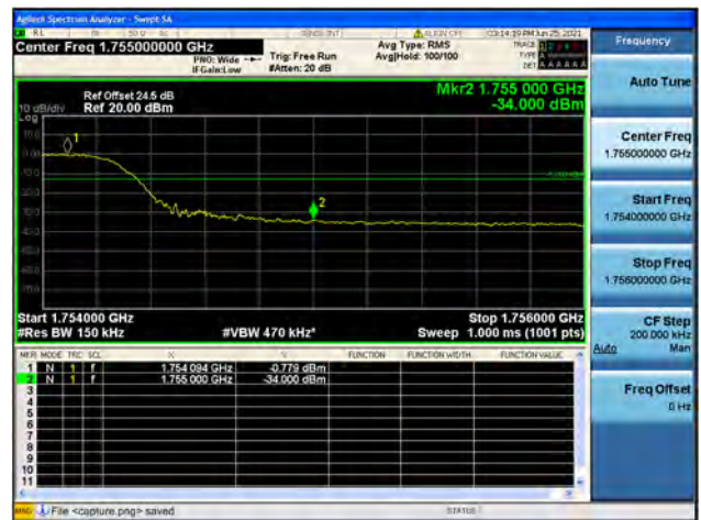
Band4 / 15MHz / High CH / QPSK / FULL RB
