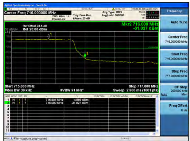
Band12 / 1.4MHz / High CH / QPSK / FULL RB
