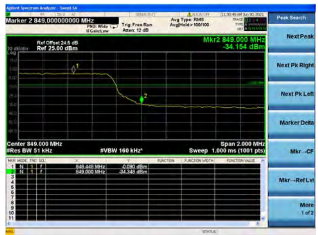
Band26 / 5MHz / High CH / QPSK / FULL RB
