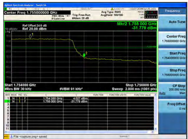
Band4 / 1.4MHz / High CH / QPSK / FULL RB
