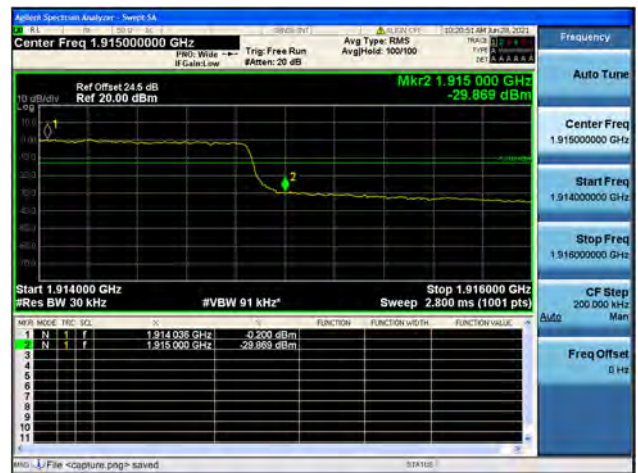
Band25 / 3MHz / High CH / QPSK / FULL RB
