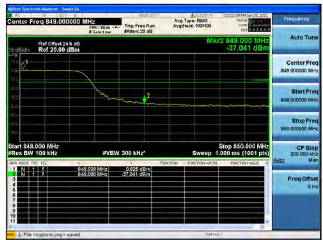
Band5 / 10MHz / High CH / QPSK / FULL RB
