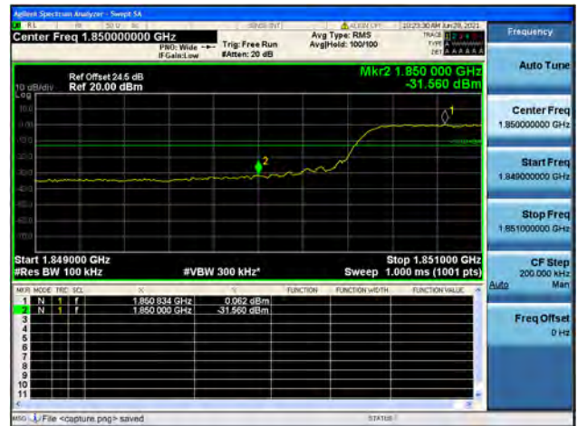
Band25 / 10MHz / High CH / QPSK / FULL RB
