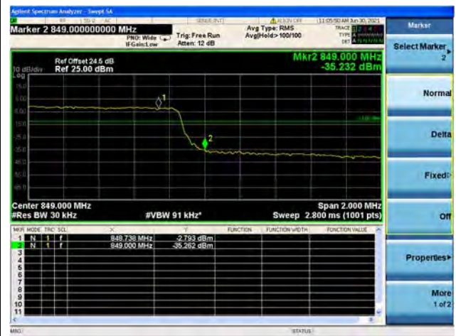
Band26 / 3MHz / High CH / QPSK / FULL RB
