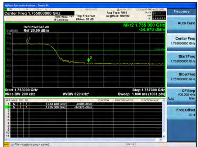
Band4 / 20MHz / High CH / QPSK / FULL RB
