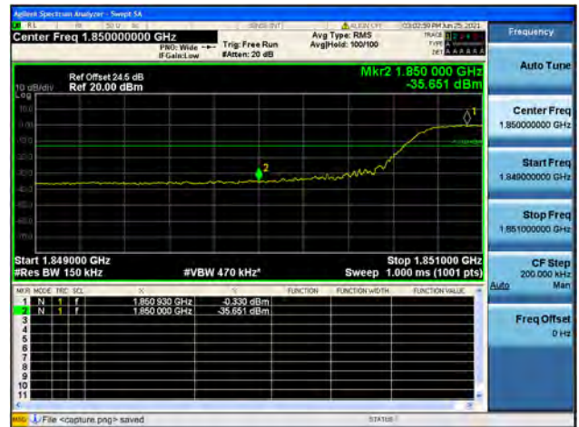
Band2 / 15MHz / High CH / QPSK / FULL RB
