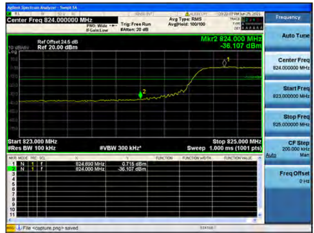
Band5 / 10MHz / High CH / QPSK / FULL RB
