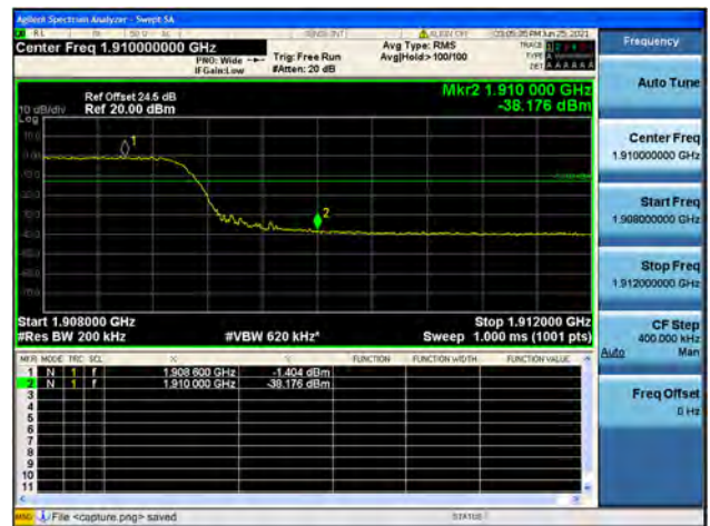
Band2 / 20MHz / High CH / QPSK / FULL RB
