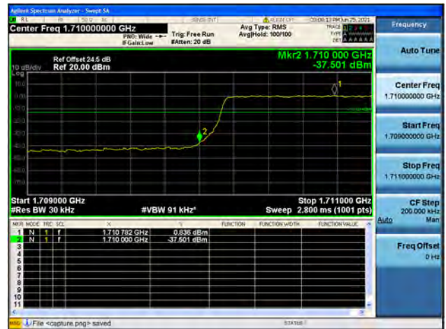
Band4 / 3MHz / High CH / QPSK / FULL RB
