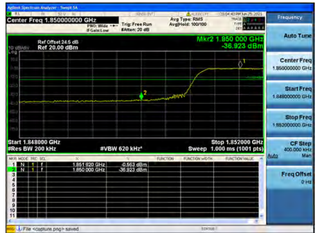
Band2 / 20MHz / High CH / QPSK / FULL RB
