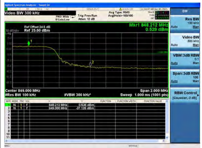
Band26 / 10MHz / High CH / QPSK / FULL RB
