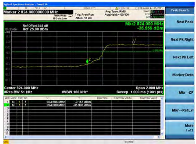
Band26 / 5MHz / High CH / QPSK / FULL RB
