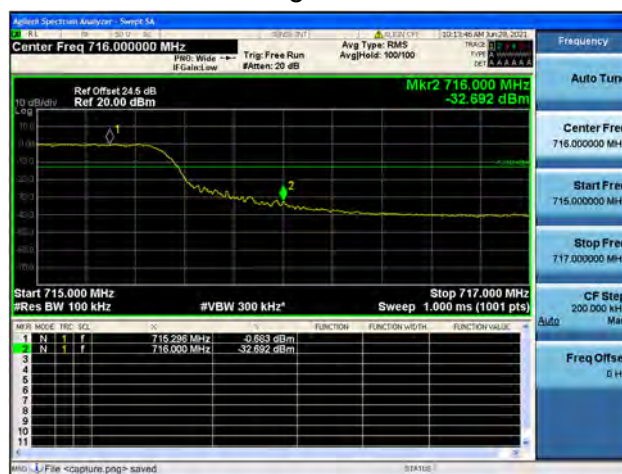
Band12 / 10MHz / High CH / QPSK / FULL RB
