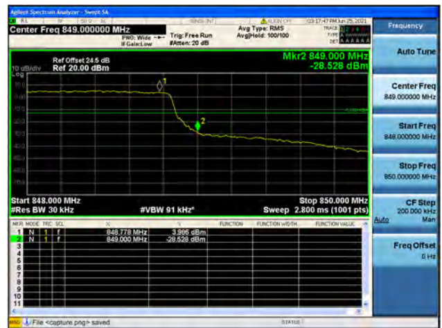
Band5 / 1.4MHz / High CH / QPSK / FULL RB
