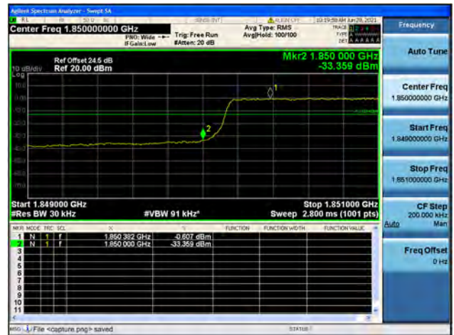
Band25 / 3MHz / High CH / QPSK / FULL RB
