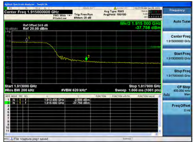
Band25 / 20MHz / High CH / QPSK / FULL RB
