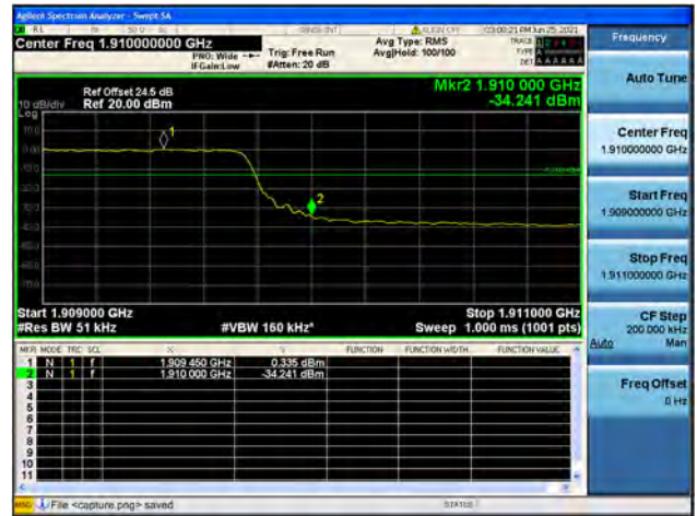
Band2 / 5MHz / High CH / QPSK / FULL RB
