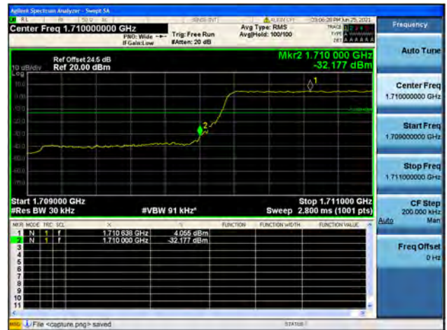
Band4 / 1.4MHz / High CH / QPSK / FULL RB
