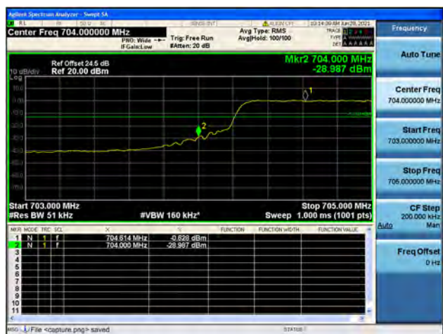
Band17 / 5MHz / High CH / QPSK / FULL RB
