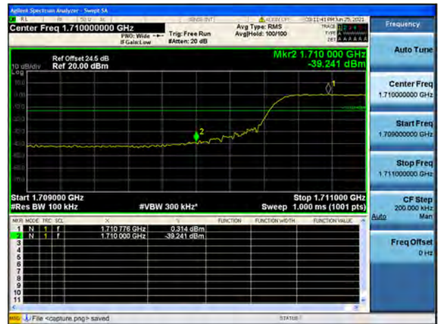
Band4 / 10MHz / High CH / QPSK / FULL RB
