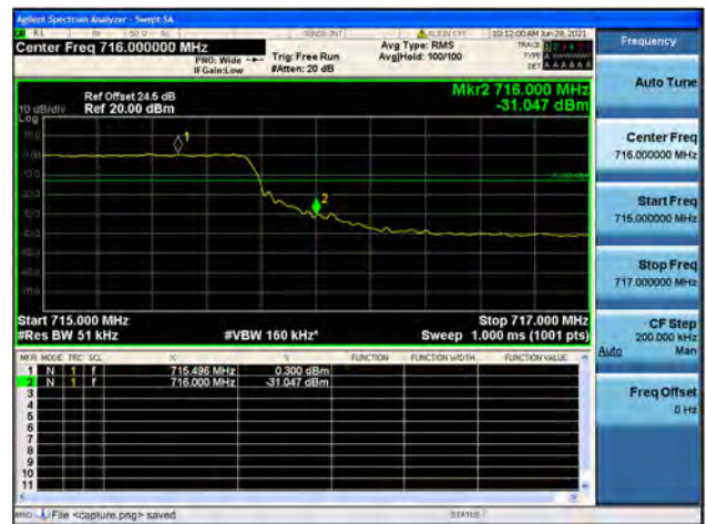
Band12 / 5MHz / High CH / QPSK / FULL RB
