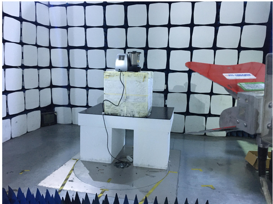
Radiation Emission Test Setup (1GHz to 18GHz)
