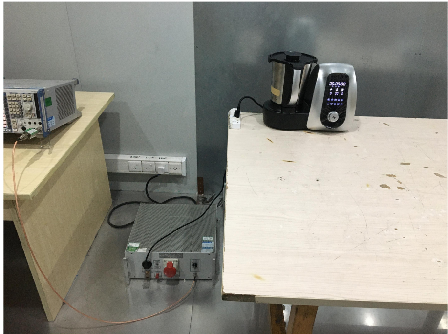
Conducted Emission Test Setup
