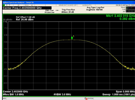
Peak Output Power BLE 1M Channel 0
