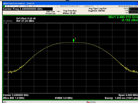
Peak Output Power BLE 1M Channel 39
