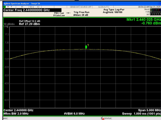
Peak Output Power BLE 2M Channel 19
