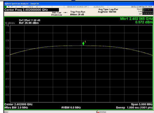
Peak Output Power BLE 2M Channel 0
