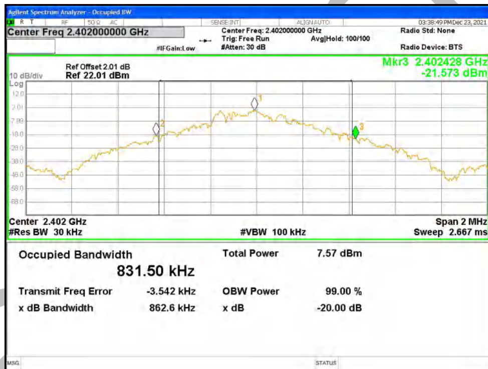
-20dB Bandwidth NVNT 1-DH1 2402MHz Ant1
