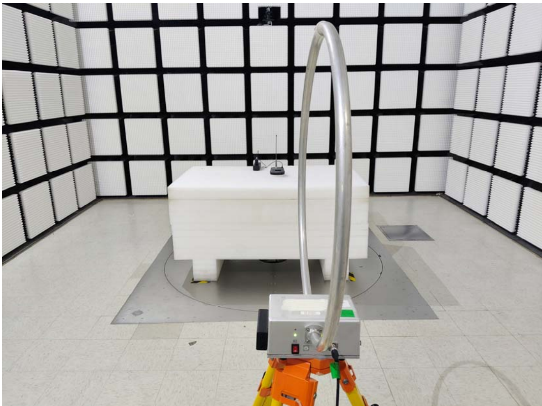
Radiated Emission 9 kHz-30 MHz Perpendicular View
