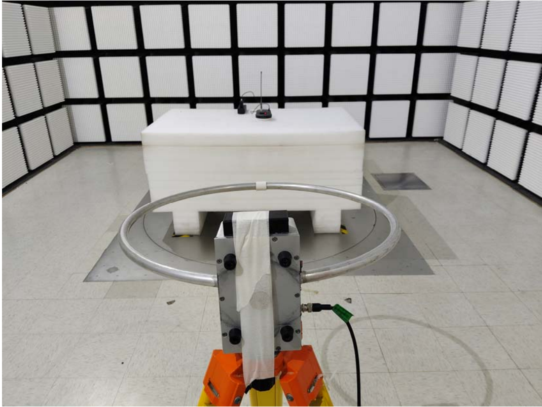
Radiated Emission 30 MHz-1 GHz View
