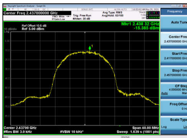
Power spectral density-802.11g ,2412MHz
