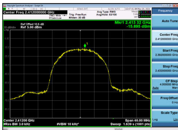
Power spectral density-802.11b ,2462MHz
