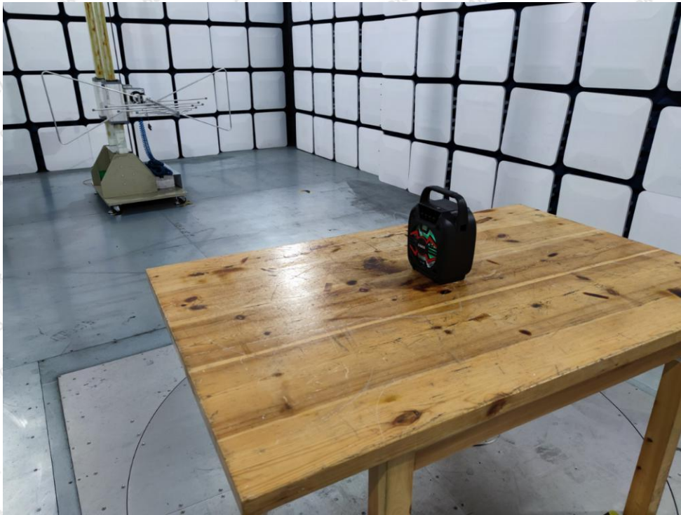
Photo of Radiation Emission Test
