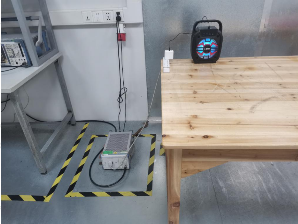
Photo of Conducted Emission Measurement
