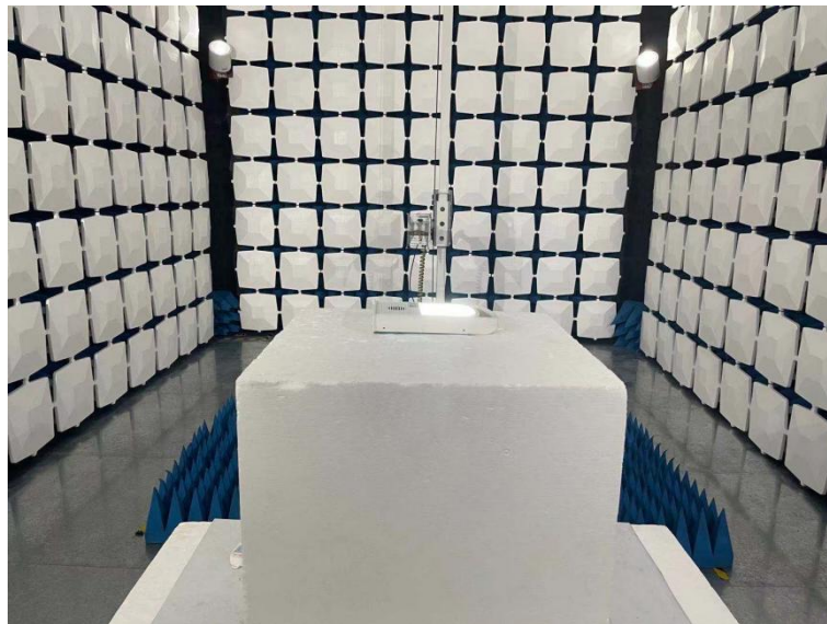
Below 1GHz for radiated emission test setup
