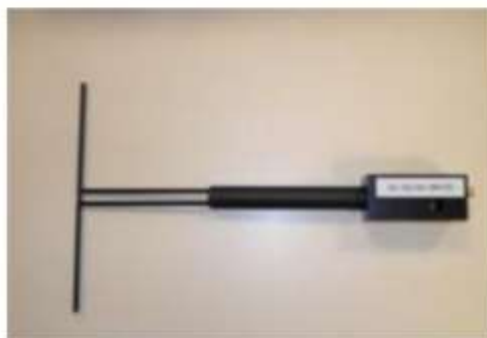
Figure 1 – Satimo COMOSAR Validation Dipole
