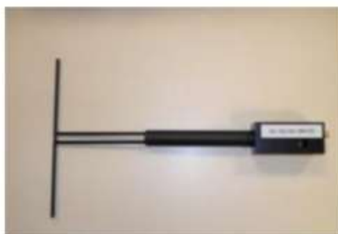
Figure 1 – Satimo COMOSAR Validation Dipole
