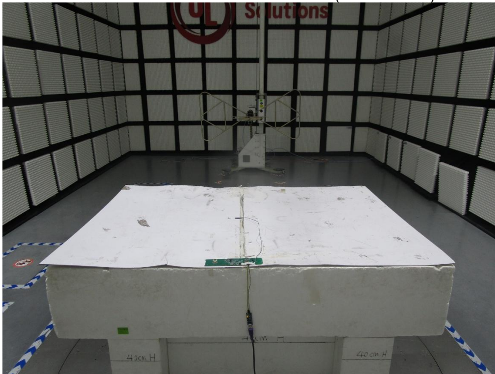
RADIATED RF MEASUREMENT SETUP (30MHz~1GHz)
