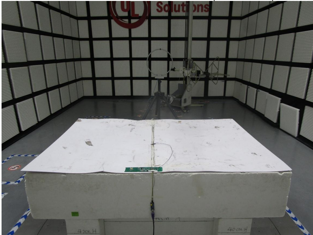
RADIATED RF MEASUREMENT SETUP (Below 30MHz)
