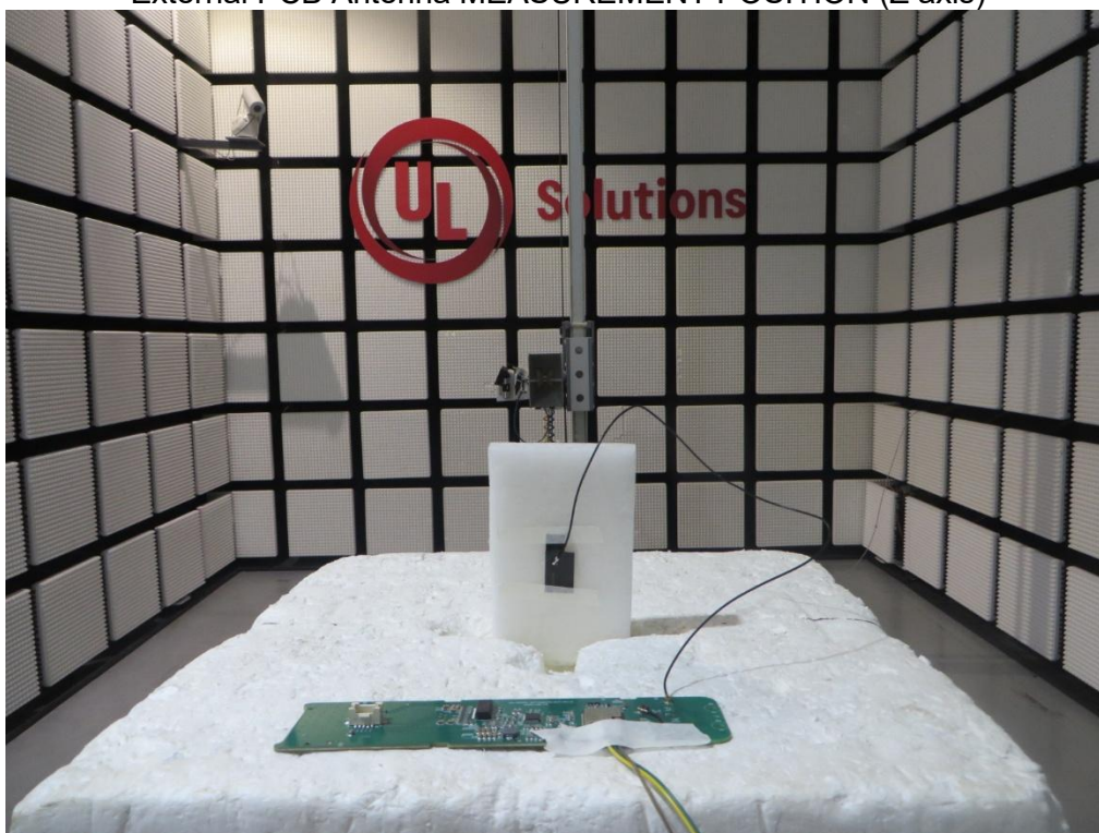
External PCB Antenna MEASUREMENT POSITION (Z axis)
