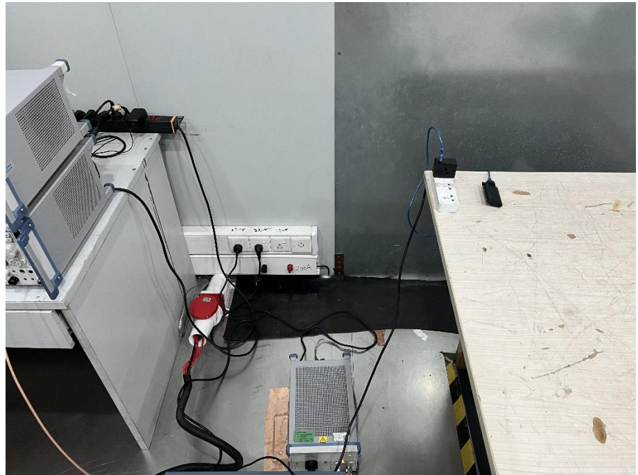
Conducted Emission Test Setup
